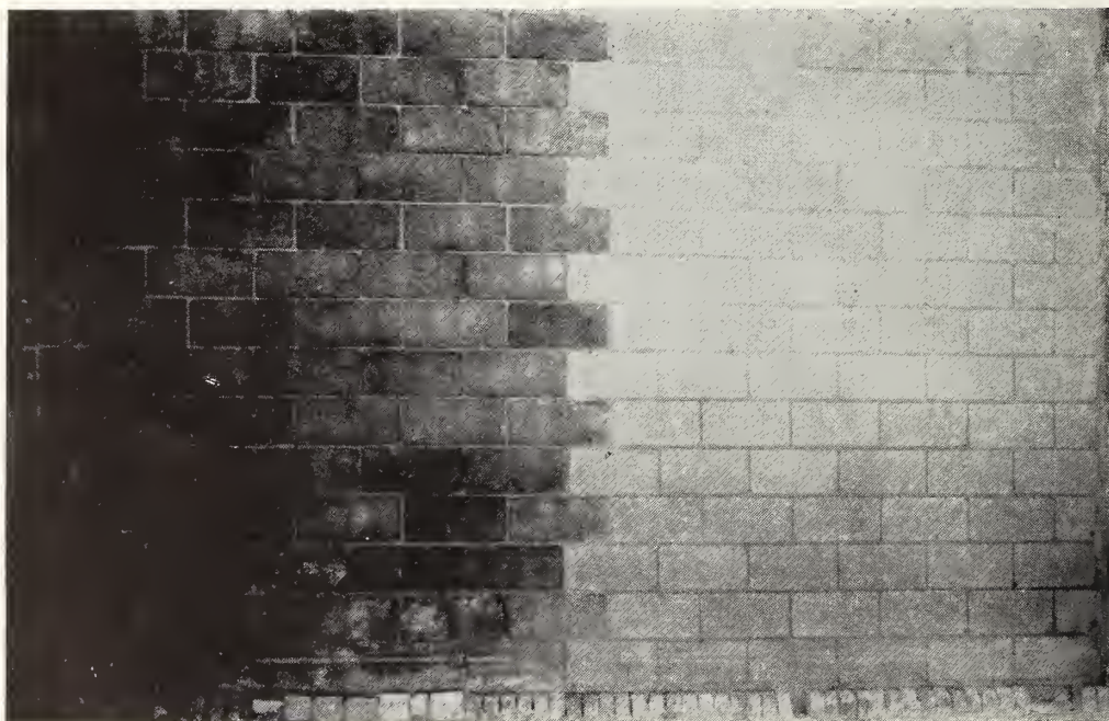
FIGURE 8. Exposed side of 6-in. nonbearing partition, 8, after fire and hose-stream tests. Cinder aggregates were used in the dark-colored and expanded-slag II aggregates for the light-colored units.
