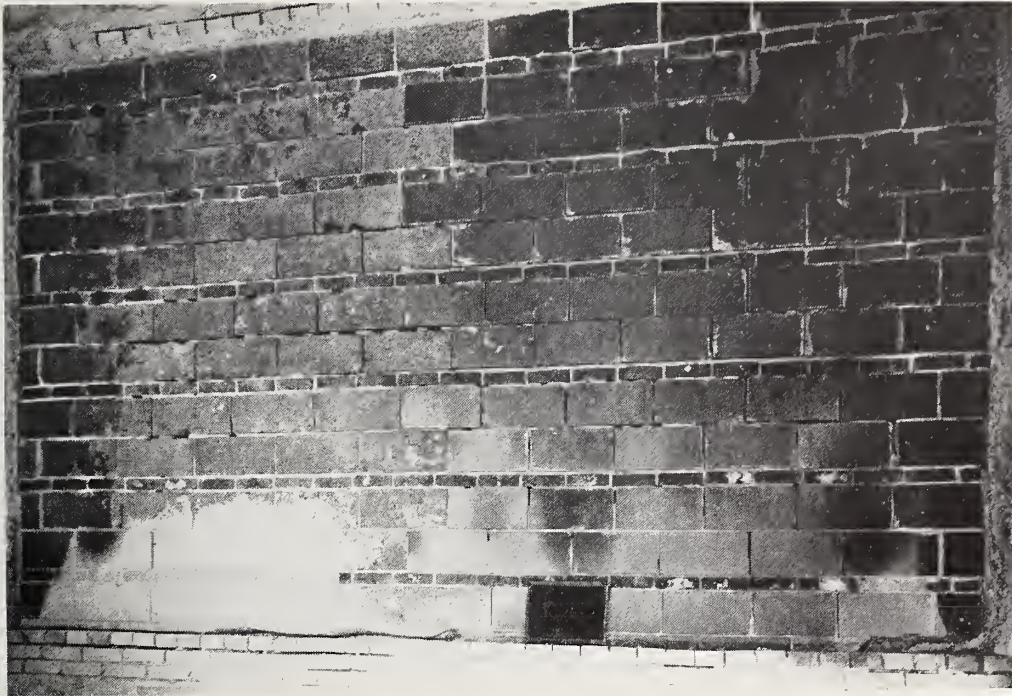
FIGURE 9. Exposed side of 8½-in. brick-faced wall, 14, after fire and hose-stream tests.
