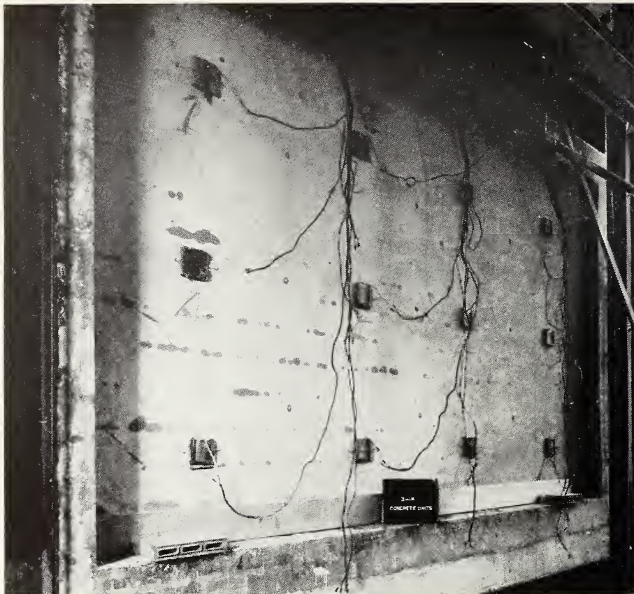
FIGURE 7. Unexposed side of nonbearing partition, 1, after 1 hr 12 min of fire exposure on the opposite side. The dark spots were caused by condensation of steam in the plaster.
