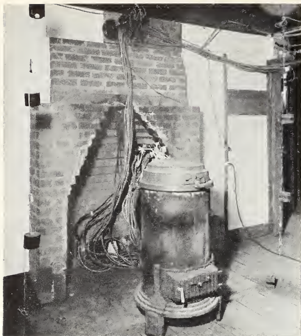
FIGURE 6. Heater A in position 2 with unattached fan mounted near the ceiling above the mantel.
