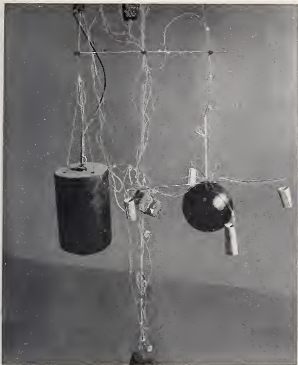
FIGURE 14. View showing globe thermometer, shielded thermocouples, cork-covered thermocouples, and an enclosed mercury element for a temperature recorder.
