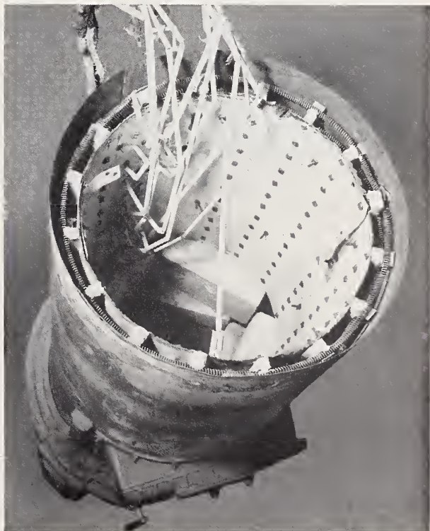
FIGURE 11. Heater A with dome removed showing position of electric heating element in the heater.
