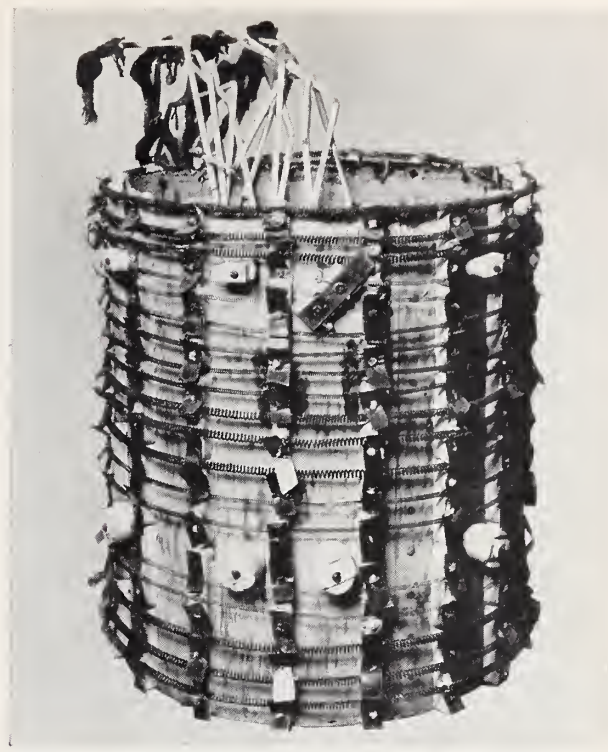
FIGURE 10. Electric heating element used for tests with heaters A and B.
