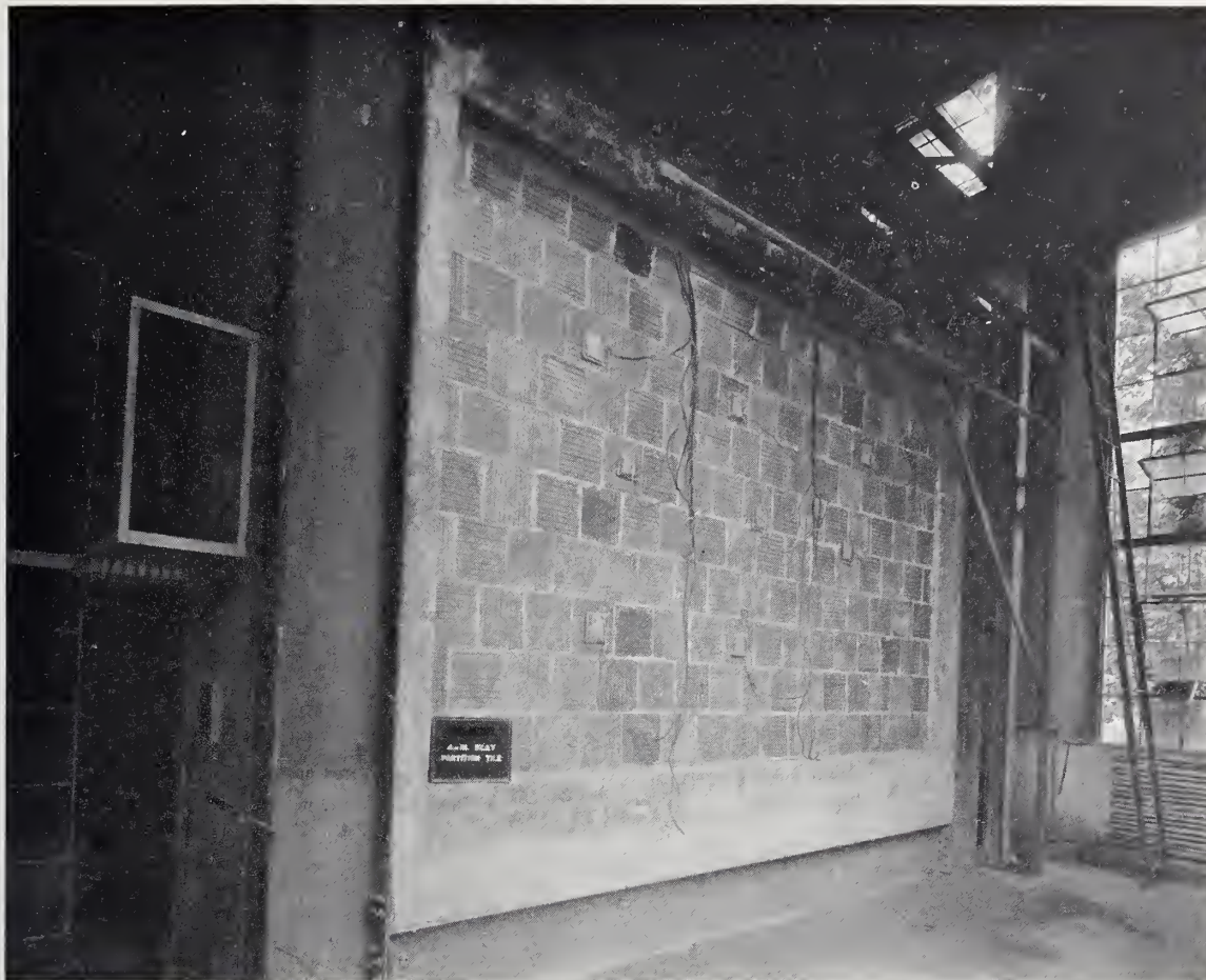
FIGURE 3. Partition 4 in furnace after a fire exposure of 12\frac{1}{2} min, on the opposite side. The restraining frame, observation windows, and asbestos pads for protecting thermocouples are shown.
