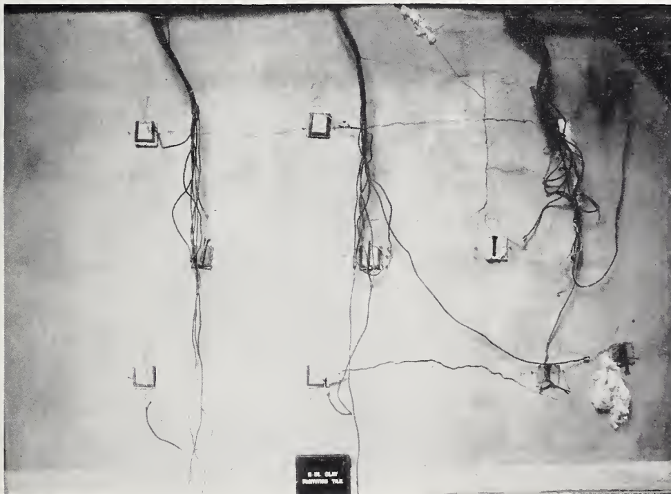
FIGURE 9. Unexposed side of partition 19 showing cotton waste which ignited at 1 hr 50 min.
