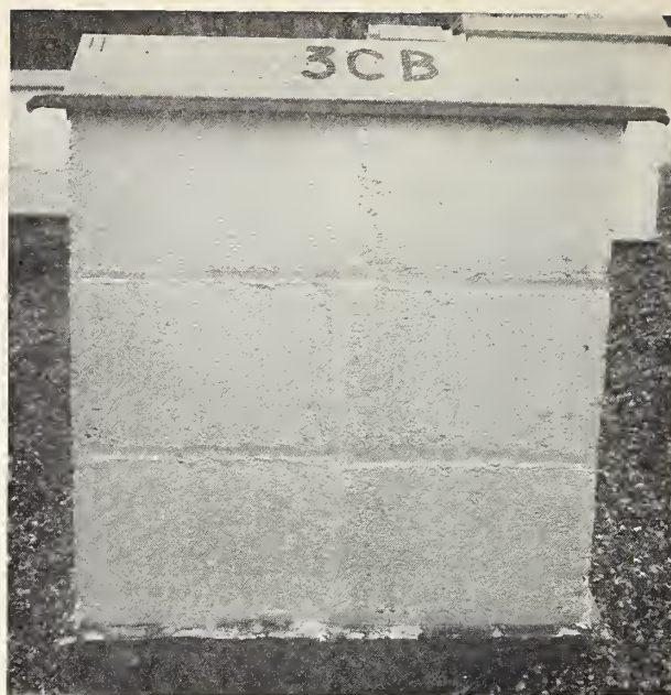
FIGURE 7.—Resin-emulsion paint, RE-1, applied over portland cement wash to stone-concrete block.
