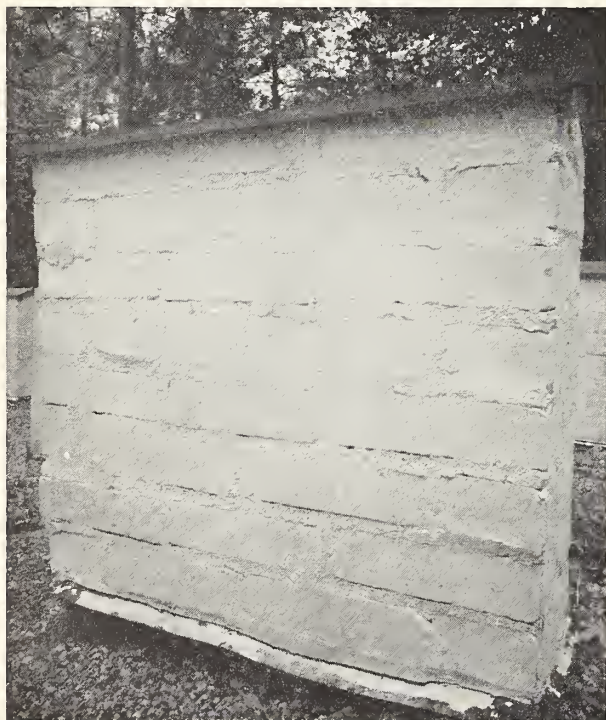
FIGURE 3.—Specimen of new common brick painted with two coats of commercial cement-water paint.
