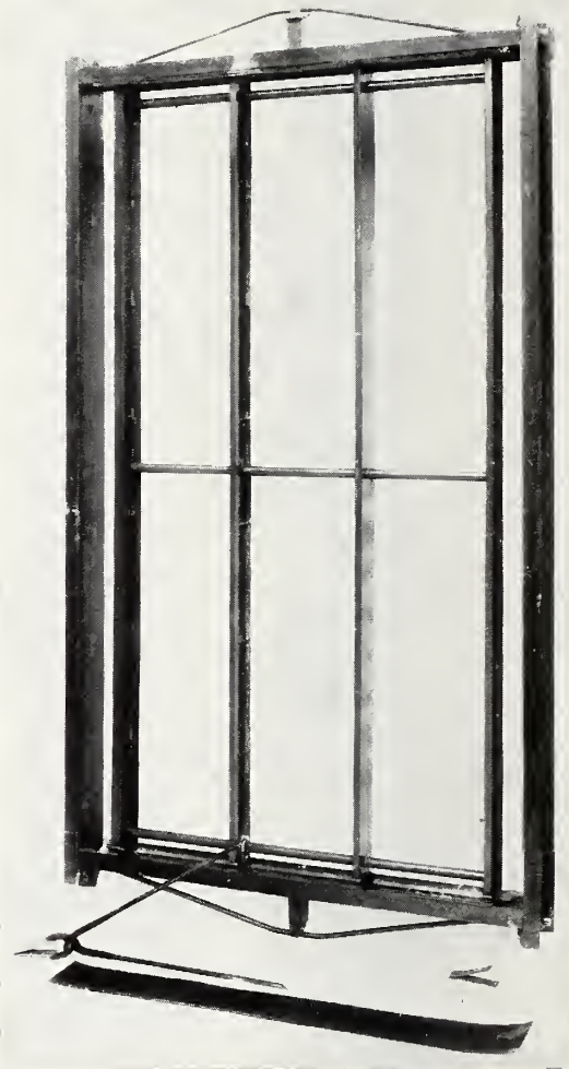
FIGURE 3.—Test frame with the frame of a wall specimen in place.
