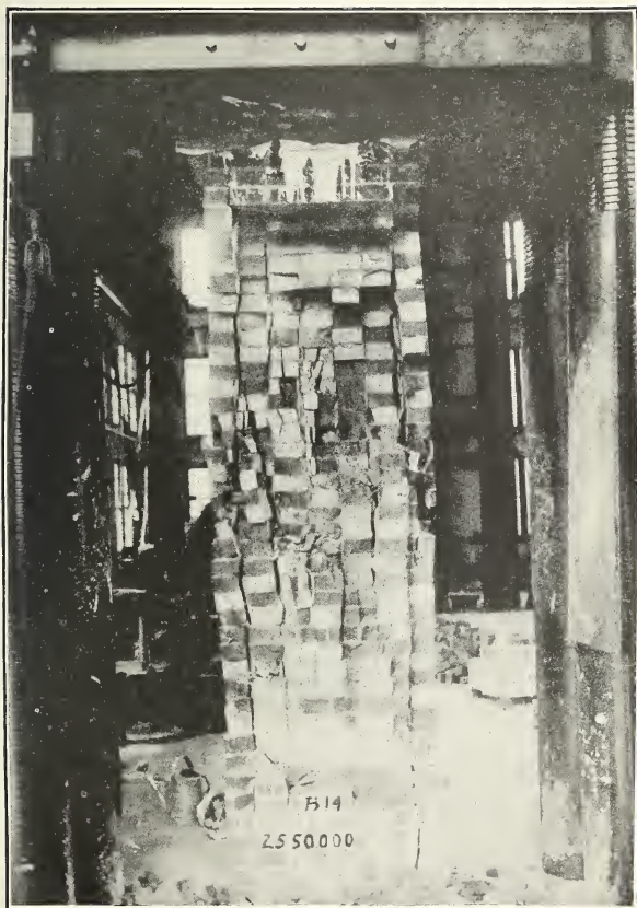
FIG. 4.—Compression test of large brick pier in 10,000,000-pound machine. Bureau of Standards laboratory at Pittsburgh
