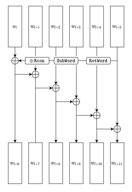
Figure 7. KEYEXPANSION() of AES-192 to generate the words w[i] for  $6 \le i < 52$ , where l ranges over the multiples of 6 between 0 and 42
