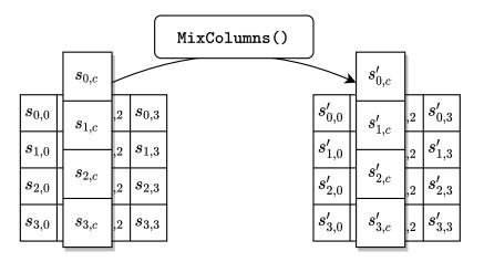
Figure 4. Illustration of MIXCOLUMNS()
