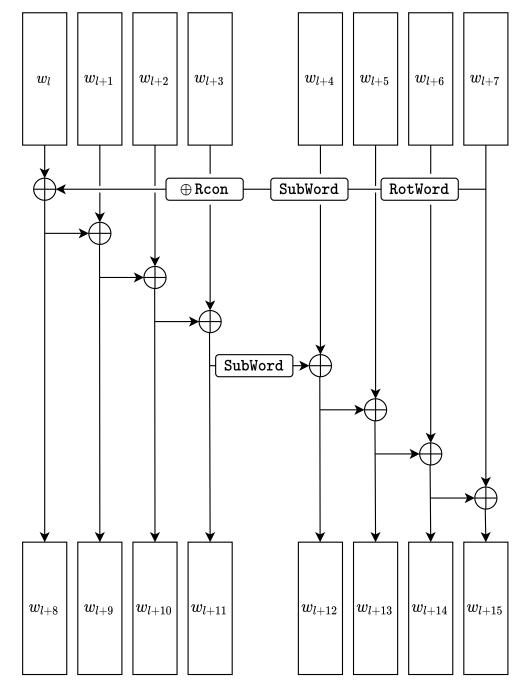
Figure 8. KEYEXPANSION() of AES-256 to generate the words w[i] for  $8 \le i < 60$ , where l ranges over the multiples of 8 between 0 and 48
