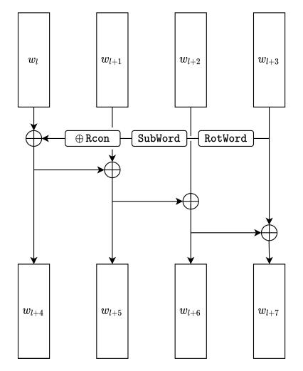
Figure 6. KEYEXPANSION() of AES-128 to generate the words w[i] for  $4 \le i < 44$ , where l ranges over the multiples of 4 between 0 and 36
