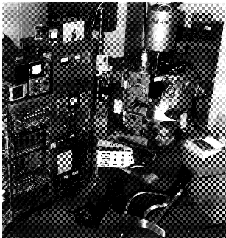
Fig. 1. Kurt Heinrich with his EMPA apparatus.
