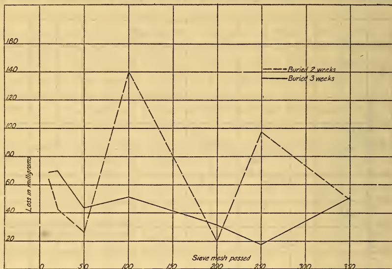
FIG. 24.—Effect of size of sand on corrosion
