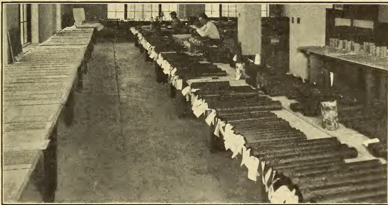
FIG. 20.—Bituminous coated materials arranged for rating
