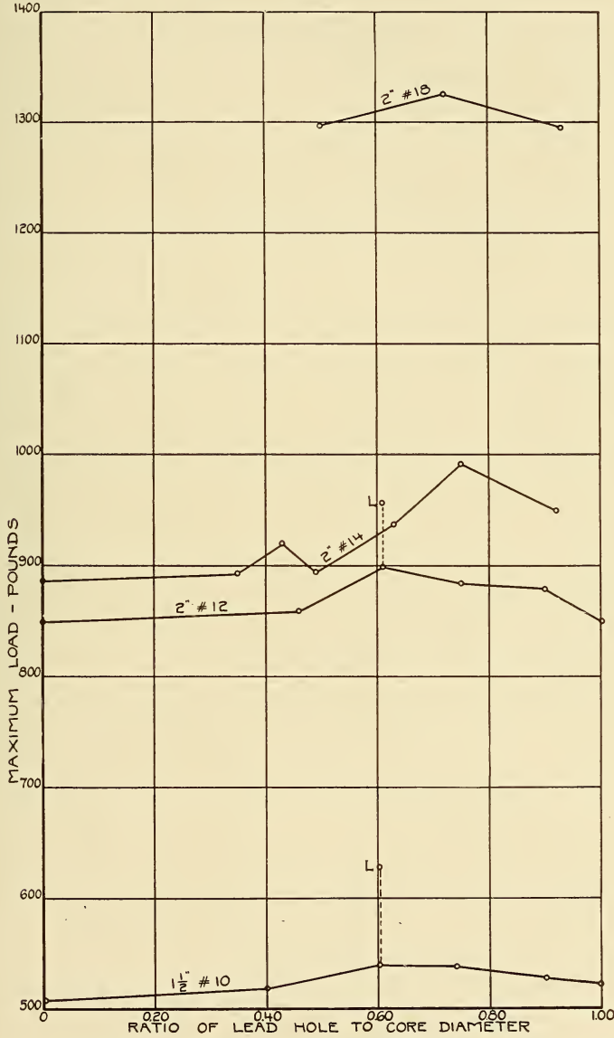
FIG. 8.—Determination of lead-hole size in sycamore
