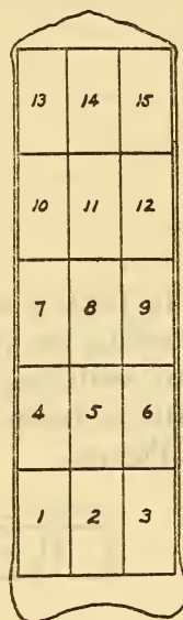
FIG. 3.—Distribution of patterns cut from railway firebox plate (Series 4 Steel)
