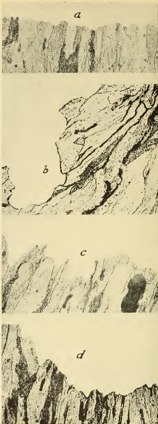
FIG. 31.—Microphotographs of the fractures of fire box boiler plate obtained at 465^{\circ}\text{C} . under different rates of loading. \times 500
