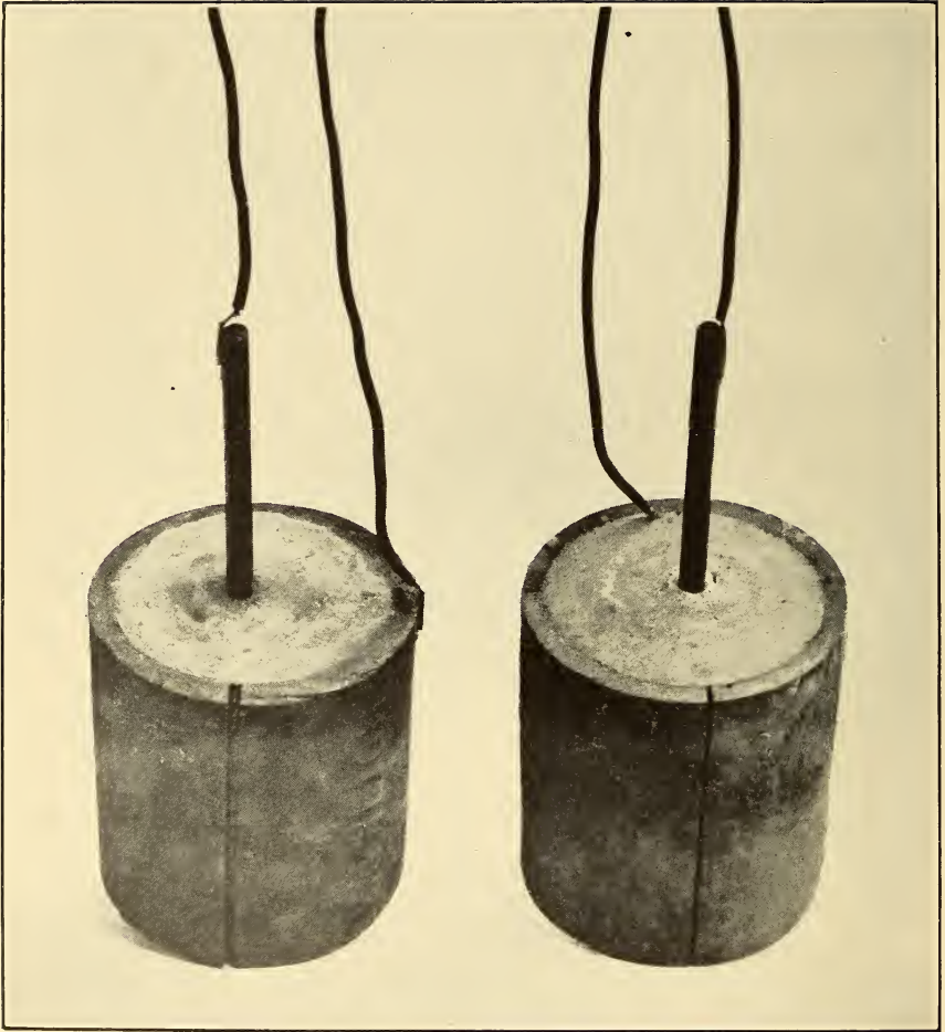
Fig. 11.—Specimens used in tests to determine the force produced by the corrosion of iron in concrete
