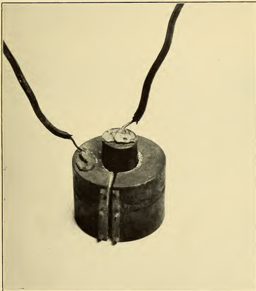
Fig. 12.— Specimen used in test to determine the force produced by the corrosion of iron in concrete
