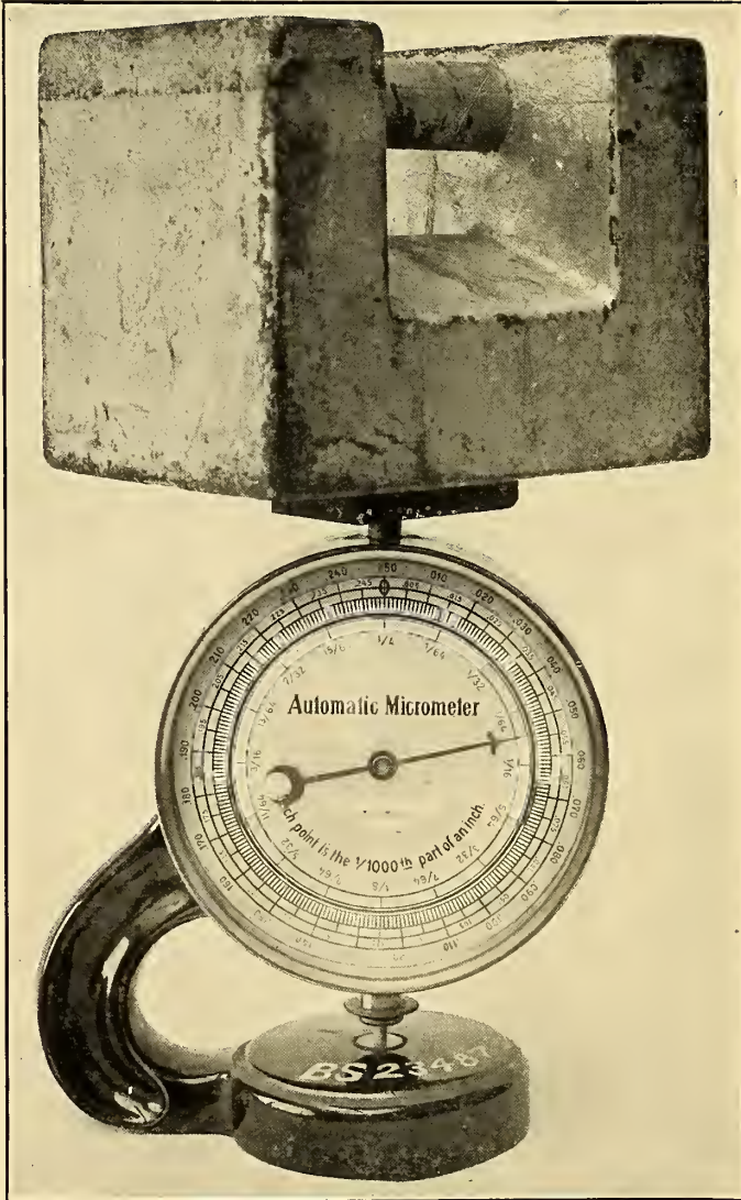
FIG. 21.—Micrometer adapted to measure flow of amalgam
