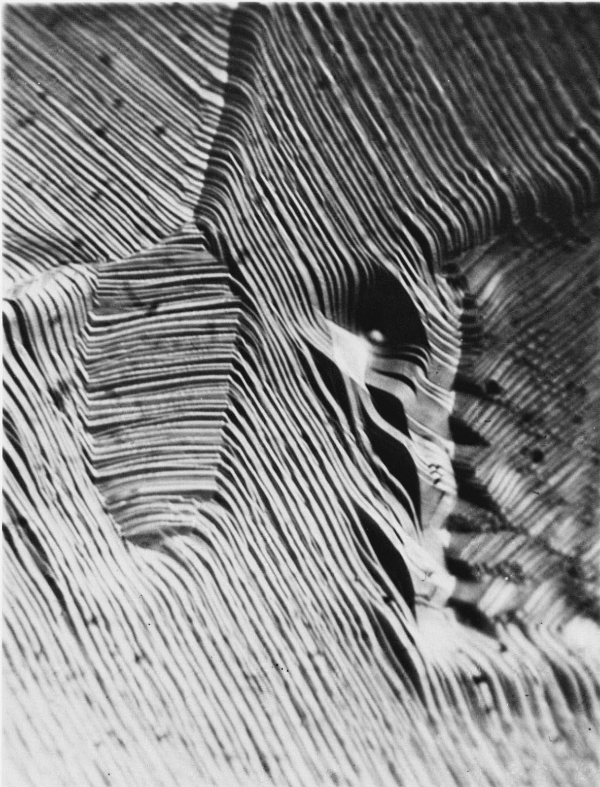
FIGURE 4. *Pure platinum crucible heated in a silicon carbide muffle furnace four hours at 1200 °C. ( $\times 2000$ )*
