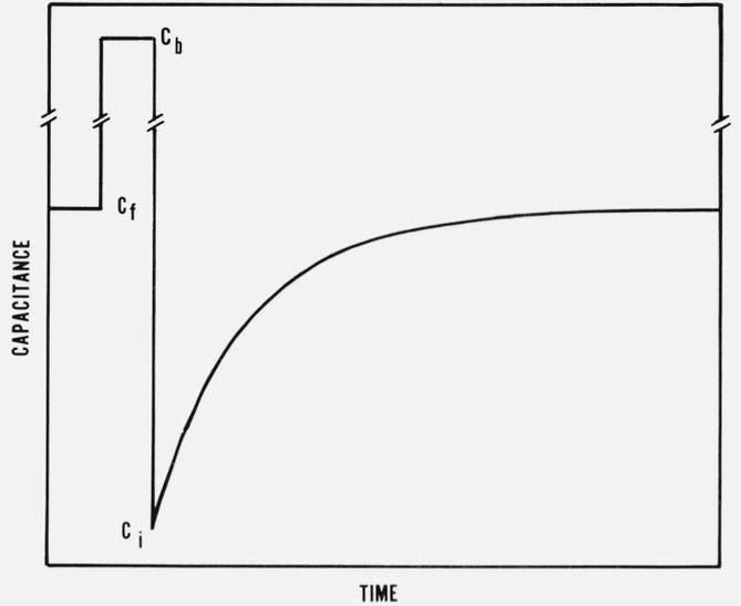
FIGURE 4. A schematic plot of the isothermal capacitance transient with the key capacitance values identified.
