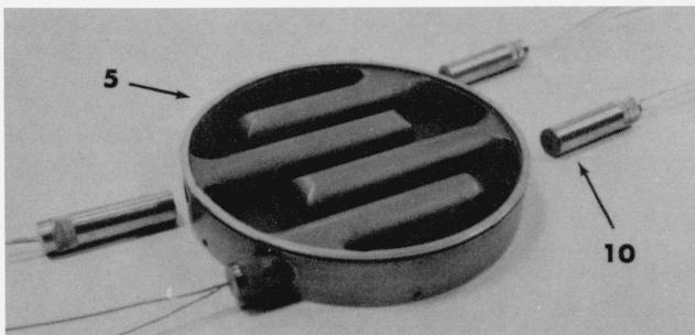
FIGURE 6. The thermal chuck assembly: (b) Inverted view of the chuck body with the heater cartridges.
