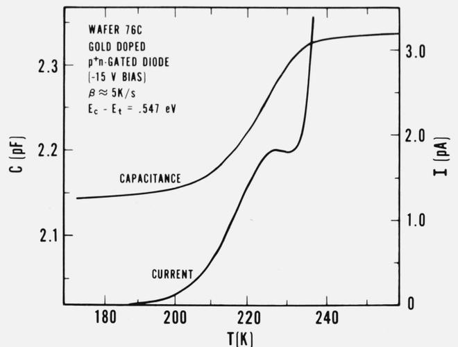
FIGURE 9. Thermally stimulated capacitance and current responses of the midgap gold acceptor (heating rate  $\approx 5 \text{ K/s}$ ).
