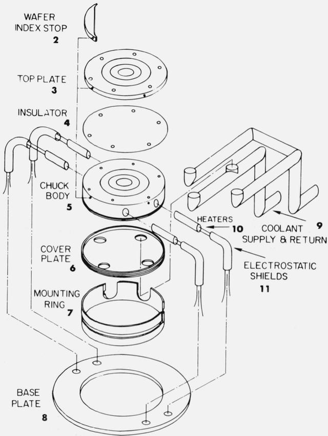
FIGURE 6. The thermal chuck assembly: (a) Detailed view of the major components.
