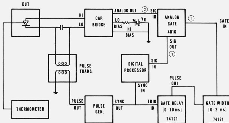
FIGURE 5. Block diagram for the modified ITCAP method for measuring the emission rate of a defect.
