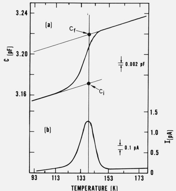
FIGURE 7. The thermally stimulated (a) capacitance and (b) current responses of a gold-doped  $n^+p$  diode (heating rate  $\approx 7\text{K/s}$ ).
