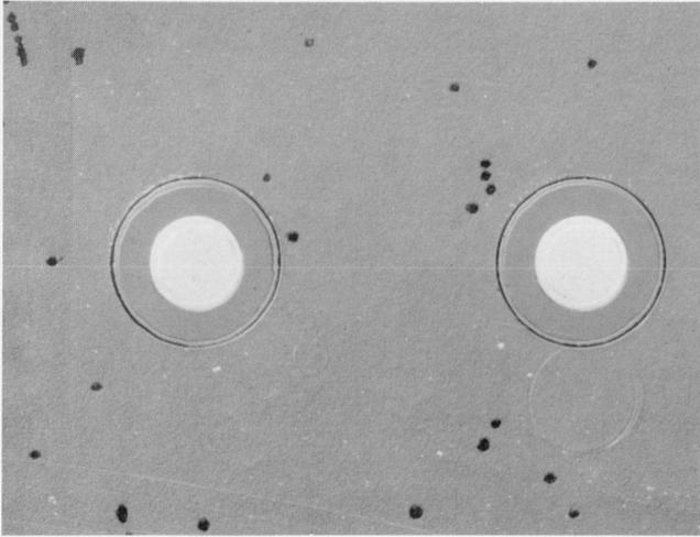
FIGURE 3. Photograph of the plasma etched mesa diode; the major diameter of the mesa is about 230  $\mu\text{m}$ .
