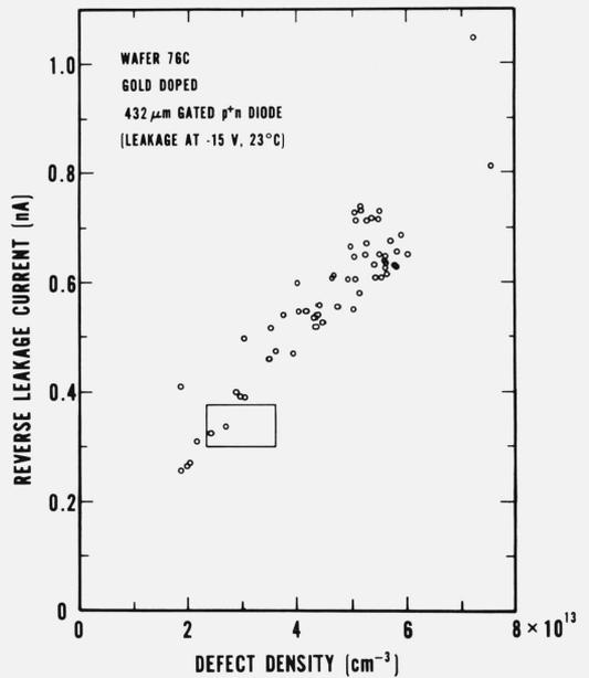
FIGURE 11. Plot of the reverse leakage current versus the acceptor defect density.
