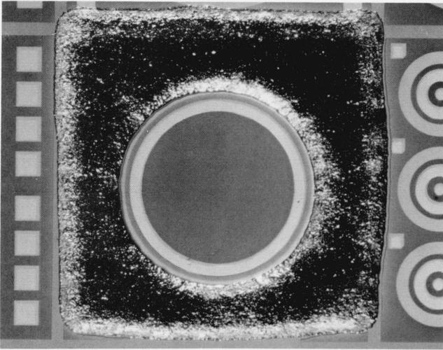
FIGURE 2. Photograph of the ultrasonically machined mesa diode; the major diameter of the mesa is about 1.5 mm.
