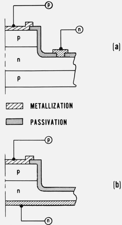
FIGURE 1. Cross sections of the proposed mesa diodes: (a) top side *n*-contact, (b) back side *n*-contact.
