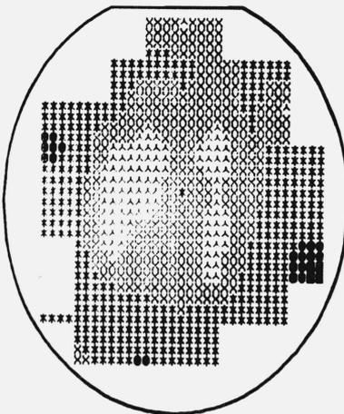
FIGURE 10. Wafer maps of (a) the gold acceptor defect density and (b) the reverse leakage current.
