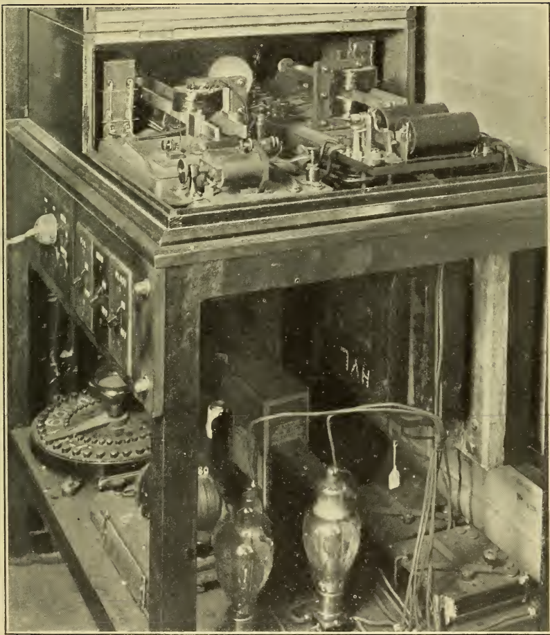
FIGURE 3.— Photograph of the assembled tuning-fork-thyratron apparatus
