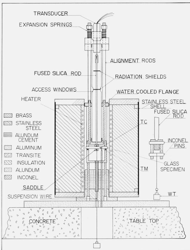
FIGURE 1. Beam-bending apparatus showing furnace and table.
