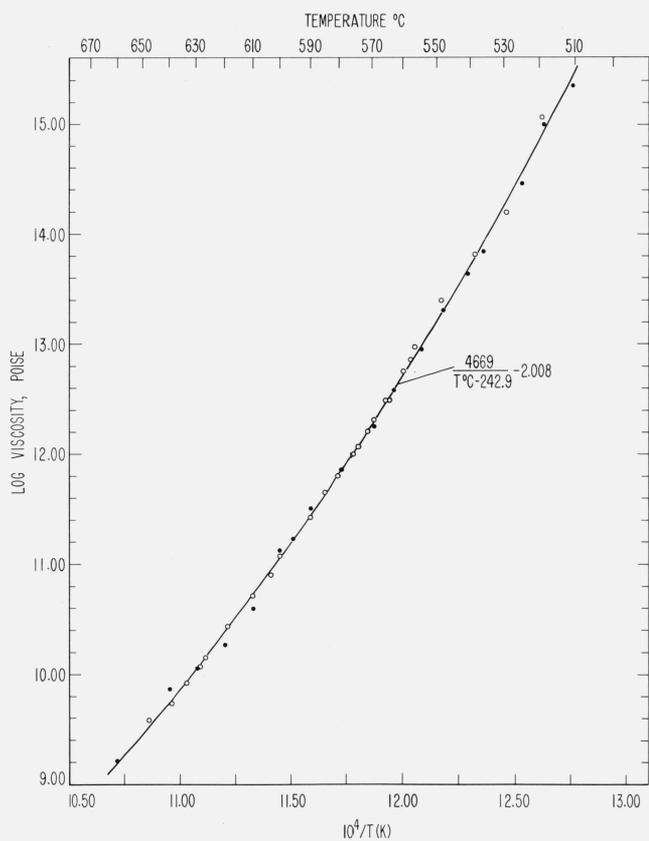
FIGURE 4. The log viscosities obtained by each method for SRM 710 compared to the equation representing the combined data from both methods.
