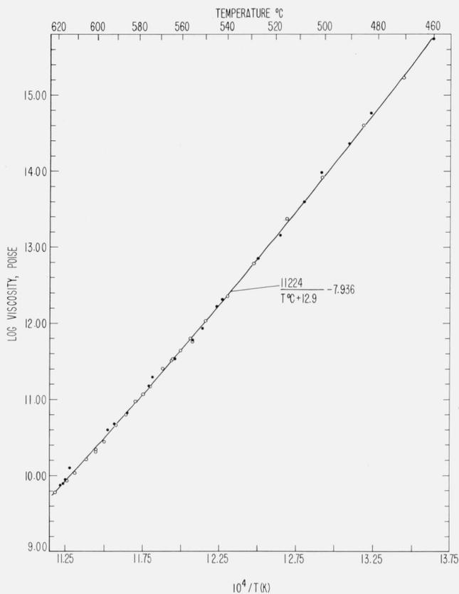
FIGURE 6. The log viscosities obtained by each method for SRM 717 compared to the equation representing the combined data from both methods.
