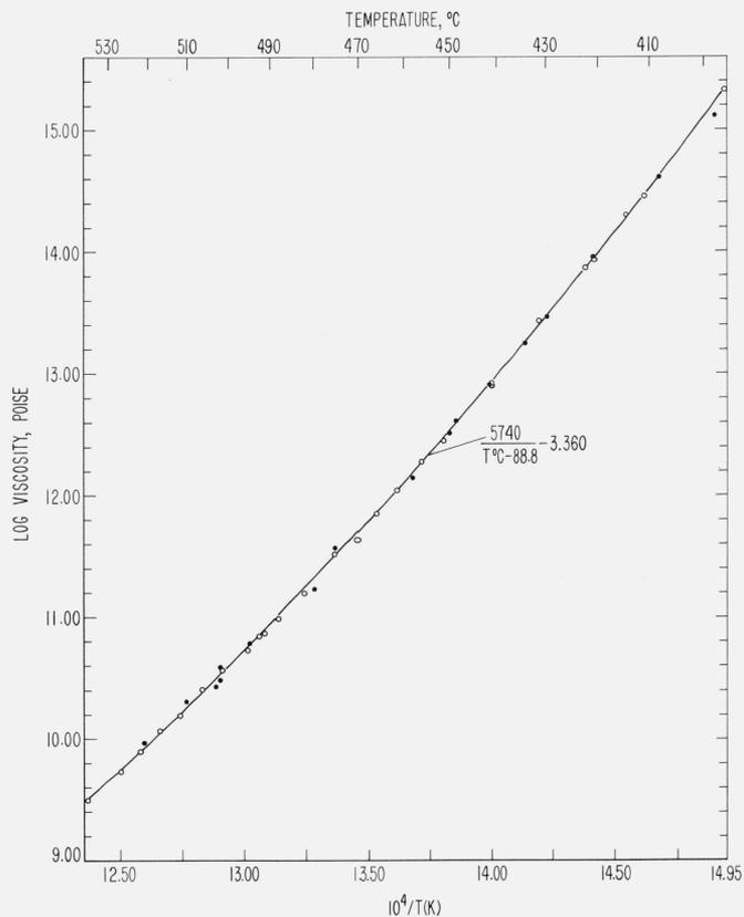
FIGURE 5. The log viscosities obtained by each method for SRM 711 compared to the equation representing the combined data from both methods.
