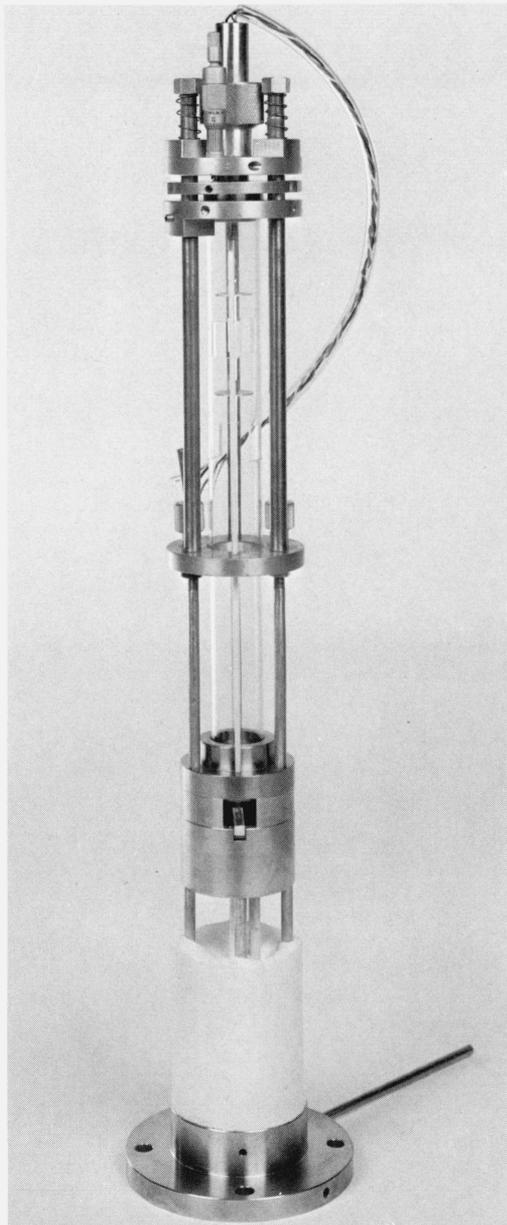
FIGURE 3. Complete beam-bending apparatus without furnace.
