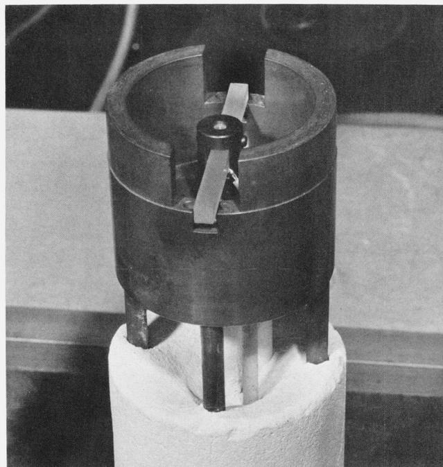
FIGURE 2. The inconel sample holder showing glass bar and saddle. Note thermocouple next to glass bar.
