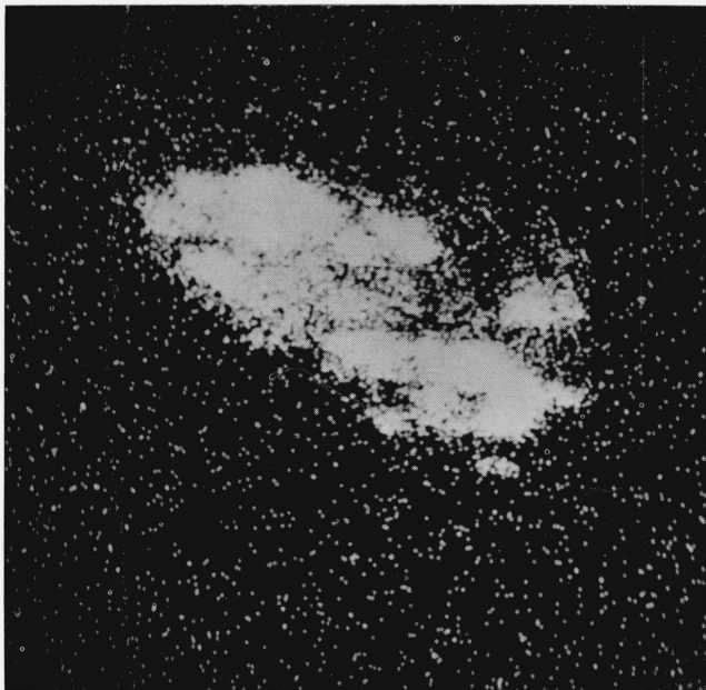
FIGURE 5. Scanning x-ray image of Ba-rich inclusions in ruby crystal, Ba L\alpha_1 , 4.6\mu/cm .
