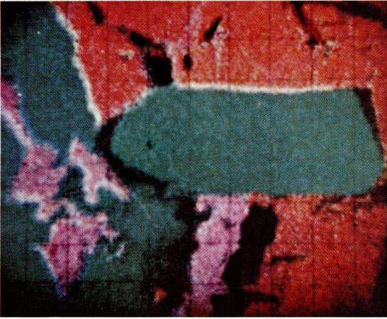
FIGURE 5d. Si green, Ag blue, S red—Si-S contrast good; Ag-S superposition has fair contrast against S; background suppressed.
