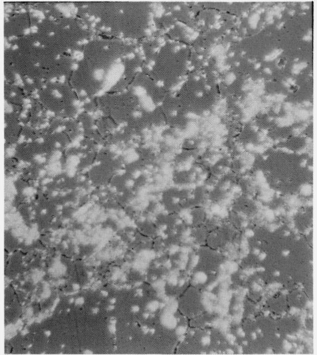
FIGURE 2. Photomicrograph taken in polarized light of composite containing 15 v/o uncoated sapphire whiskers in the as-pressed condition.
