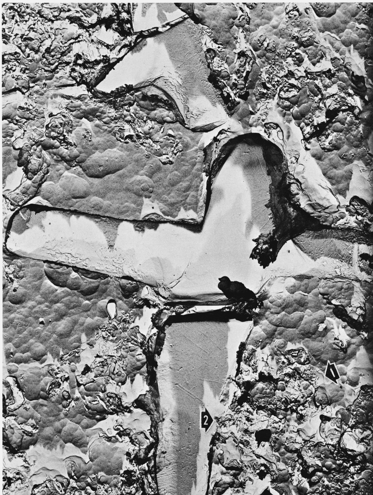
FIGURE 4. Electron micrograph of typical whisker from the same sample as shown in figure 3.
