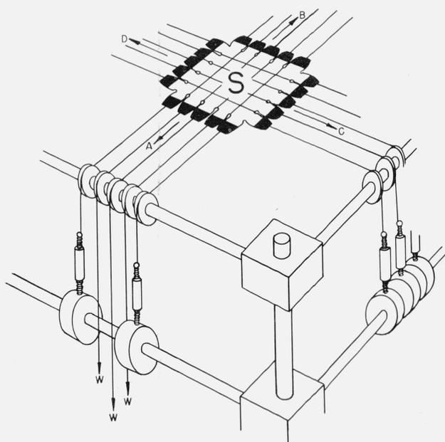
FIGURE 2. Schematic diagram for the biaxial extension experiments.
