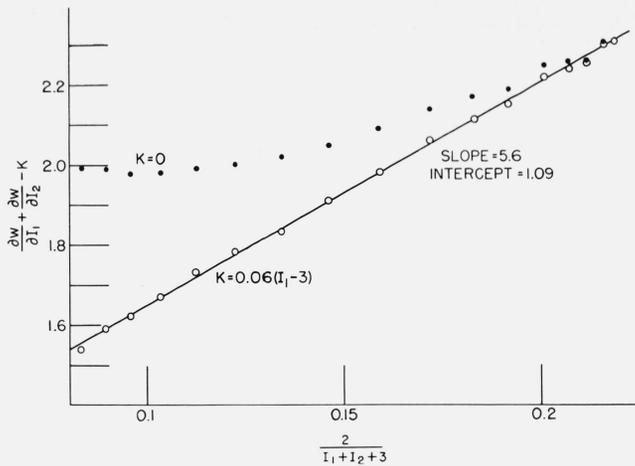
FIGURE 3. Pure shear data of Rivlin and Saunders on vulcanized natural rubber. Open circles,  $\alpha = 0$ . The abscissa is given in  $\text{kg per cm}^2$ .
