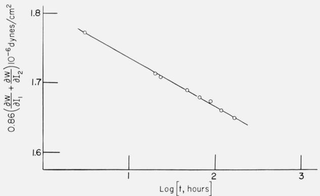
FIGURE 5. Biaxial creep data on vulcanized butyl rubber.
