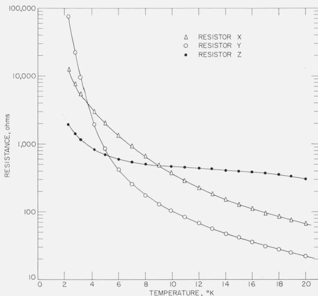
FIGURE 8. Plot of resistance as a function of temperature:  $\Delta$ , resistor X;  $\circ$ , resistor Y; and  $\bullet$ , resistor Z.
