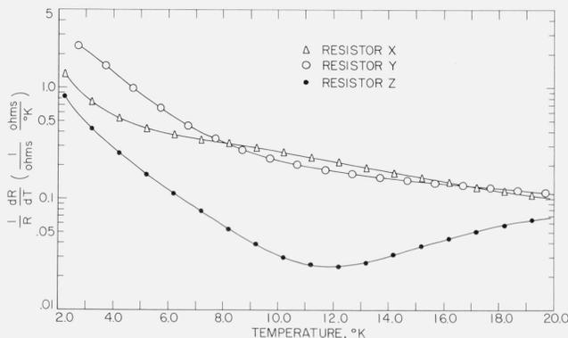
FIGURE 9. Resistance-temperature sensitivity,  $\frac{1}{R} \frac{dR}{dT} \left( \frac{1}{^{\circ}\text{K}} \right)$ , as a function of temperature ( $^{\circ}\text{K}$ ):  $\Delta$ , resistor X;  $\circ$ , resistor Y; and  $\bullet$ , resistor Z.
