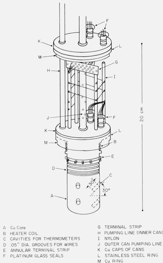
FIGURE 5. Detailed drawing of the calibrator low-temperature components.
