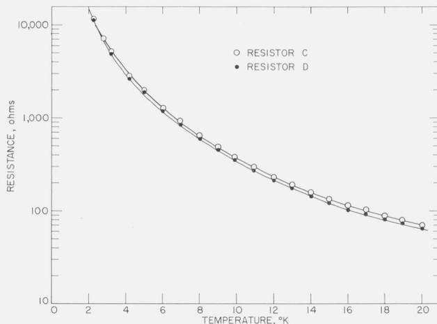
FIGURE 1. A plot of resistance as a function of temperature: ○, Resistor C; ● Resistor D.
