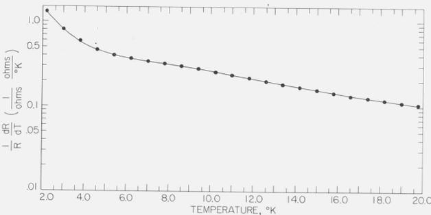
FIGURE 2. Resistance-temperature sensitivity,  $\frac{1}{R} \frac{dR}{dT} \left( \frac{1}{°K} \right)$ , as a function of temperature (°K).
