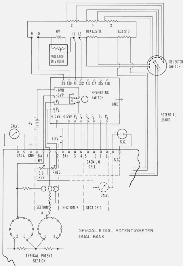
FIGURE 7. Schematic of the d-c resistance measurement circuit. This potentiometer actually consists of 3 potentiometer units in series (A, B, and C). Two sets of switches are connected to each decade to provide the "dual bank" feature.
