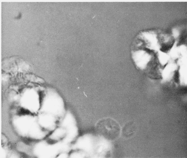
FIGURE 7. Positively birefringent spherulites and smaller aspherical aggregates grown from a 0.75 percent solution of polypropylene in mineral oil at 112 °C.
