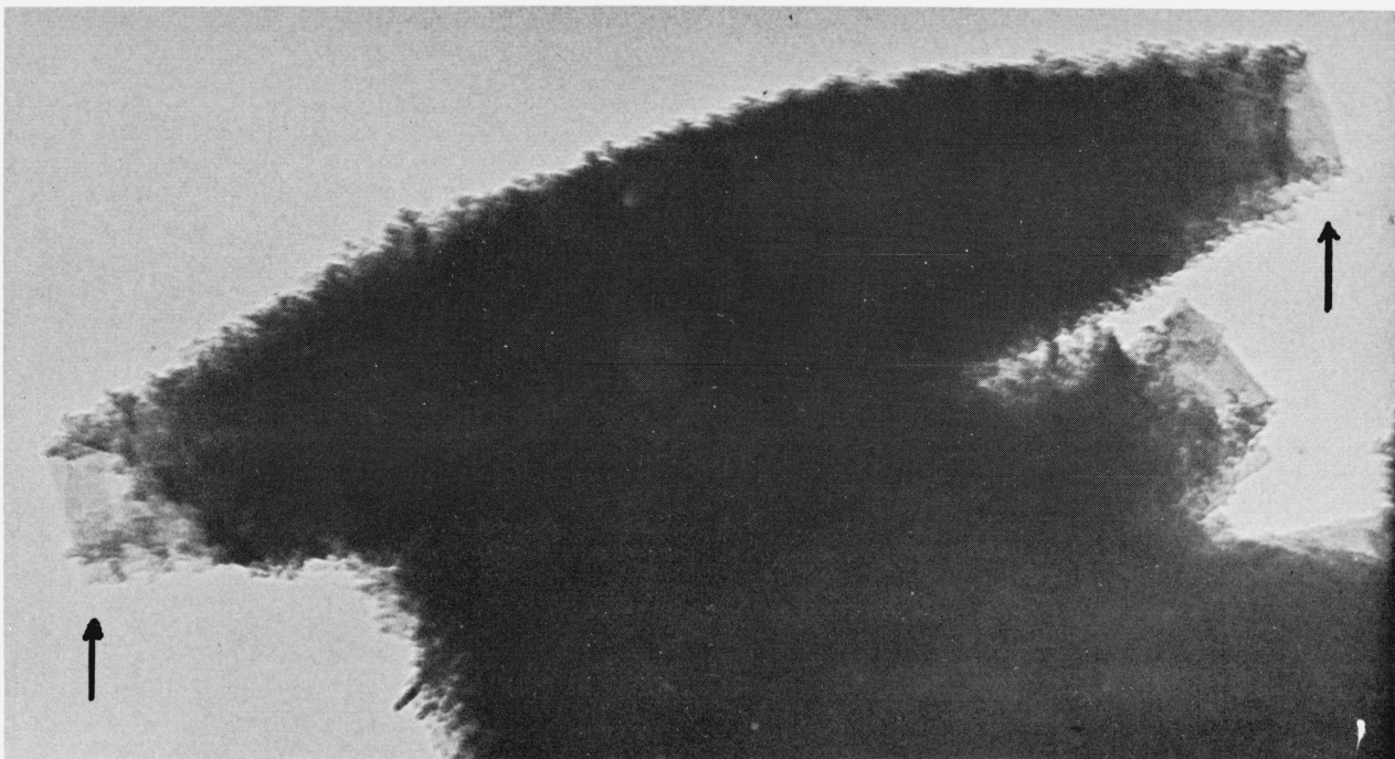
FIGURE 24. Electron micrograph of polypropylene dendrite similar to that shown in figure 23 but viewed edge-on. Note cigar shaped profile of the dendrite as well as lamellar outgrowths (arrows) protruding at both extremities. \times 53,000 .
