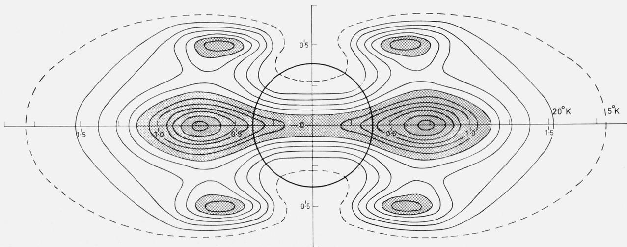
FIGURE 6. A preliminary map of the brightness distribution over Jupiter at a wavelength of 10.4 cm [Berge, 1965]. A disk component of  $280^\circ\text{K}$  has been subtracted. The contours are at intervals of  $20^\circ\text{K}$  and the angular scale (in 'arc) refers to a distance of 4.04 A.U.
