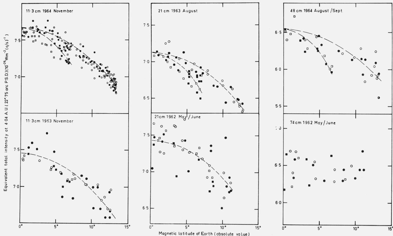
FIGURE 5. The data of figure 4 replotted as a function of the Jovomagnetic latitude of the Earth, assuming the Jovian magnetic axis is inclined  $10.0^\circ$  to the axis of rotation with the pole in the northern hemisphere at a System III longitude of  $198^\circ$ .
