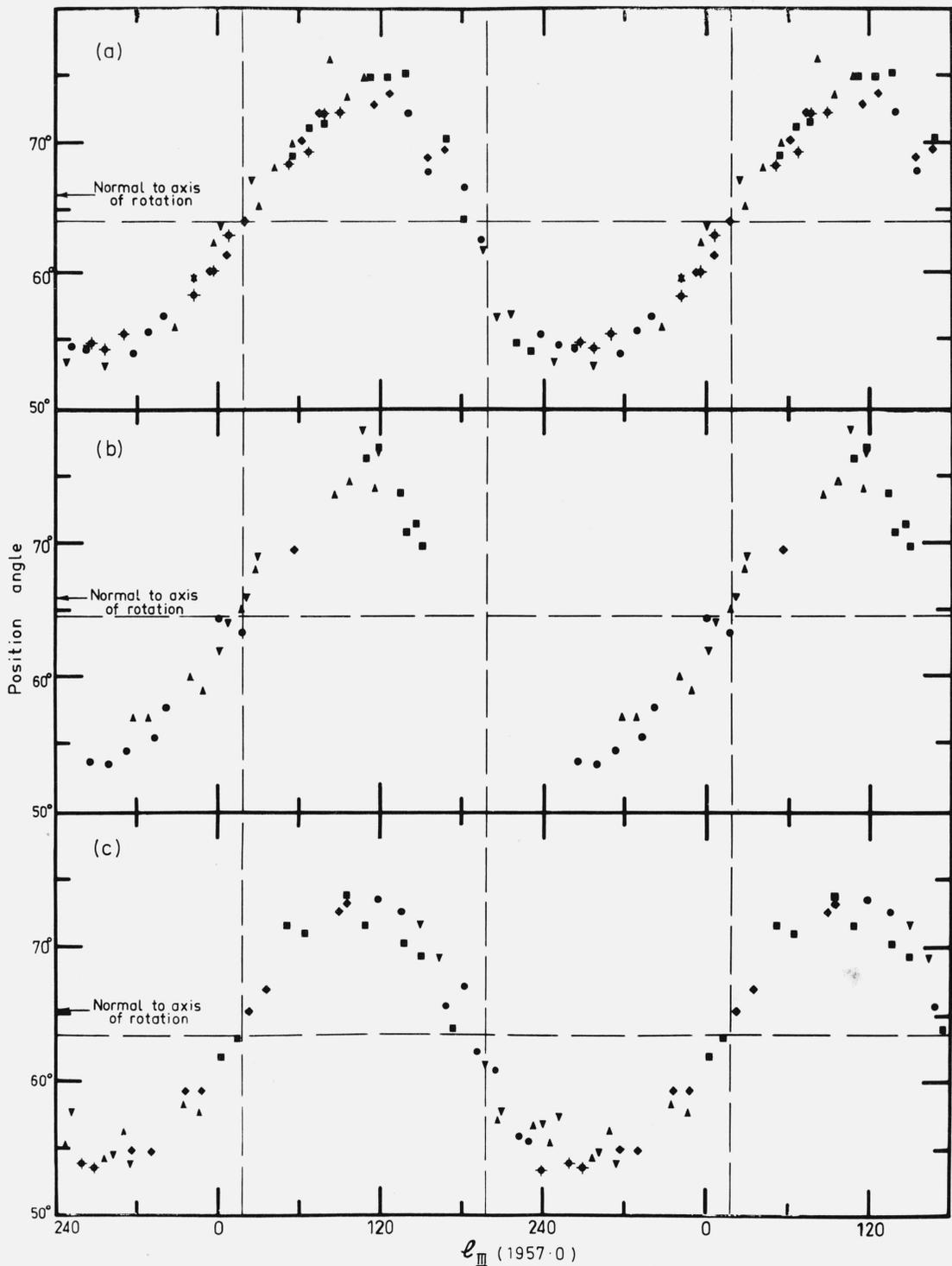
FIGURE 3. *Position angle of the maximum electric vector of the received Jovian radiation as a function of IAU System III longitude.*
