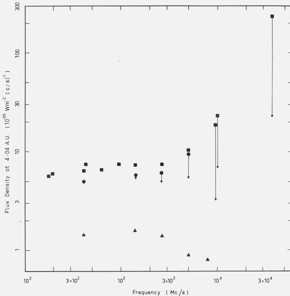
FIGURE 1. *The spectrum of the microwave emission from Jupiter at a distance of 4.04 A.U.*
