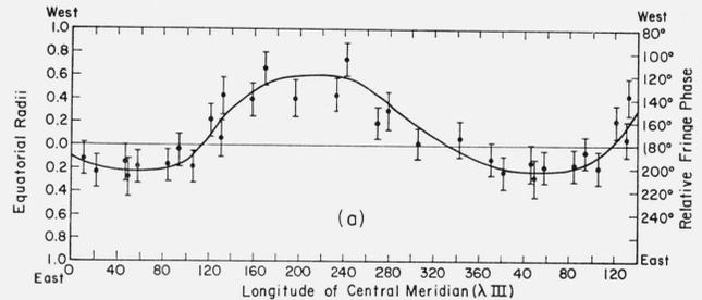
FIGURE 8a. The measurements by Berge and Morris [1964] of the relative phase of the fringes observed with an interferometer with cross-polarized and parallel polarized feeds.
