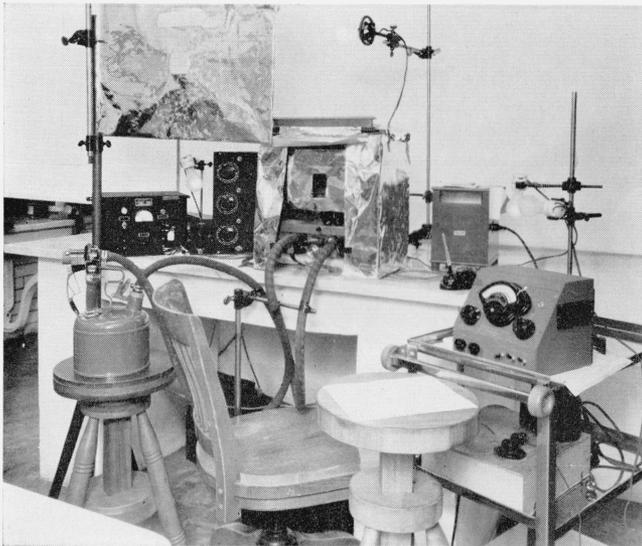
FIGURE 3. Apparatus for thermal studies and for tests for balance response to relative humidity [1].
