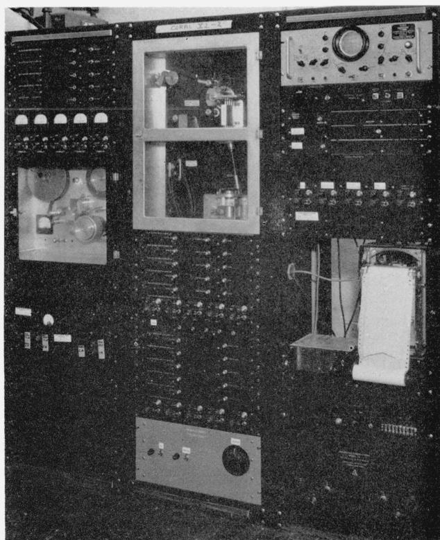
FIGURE 1. Front view of the automatic multichannel correlator.
