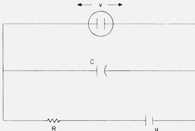
FIGURE 1. Diagram of the electric circuit.
