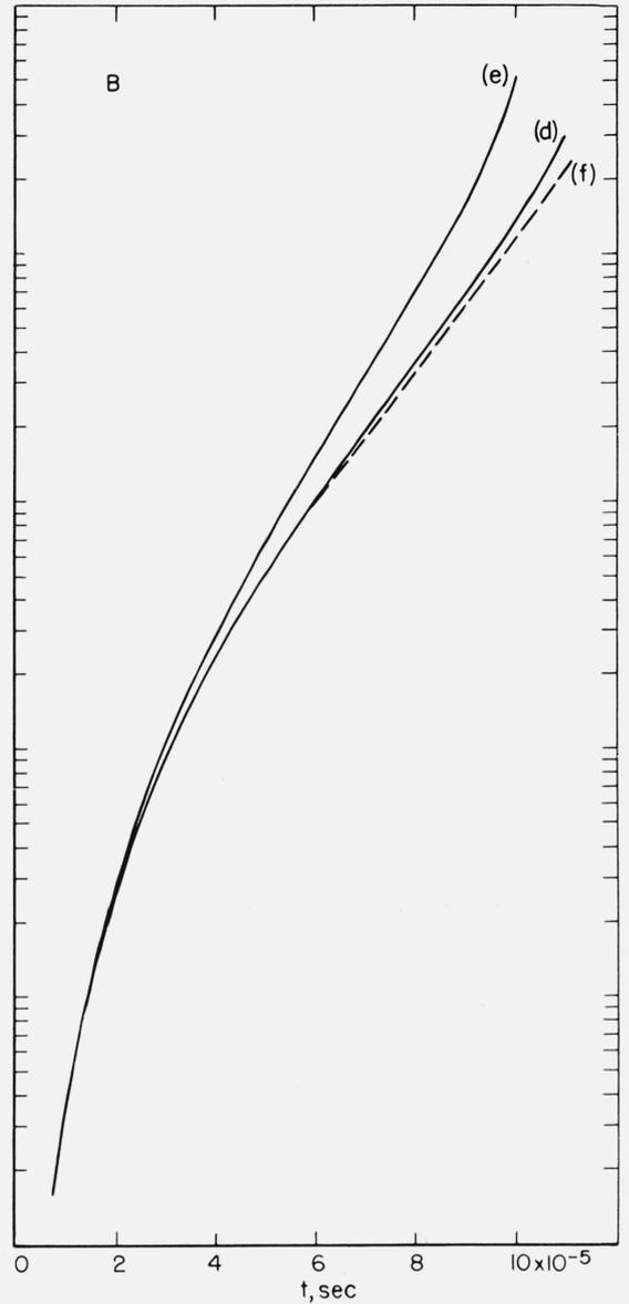
FIGURE 2B. Mean current density  $J$  across the gap versus time  $t$  for  $\gamma_p=1.5 \cdot 10^{-6}$ ,  $\gamma_i=1.35 \cdot 10^{-5}$ .
