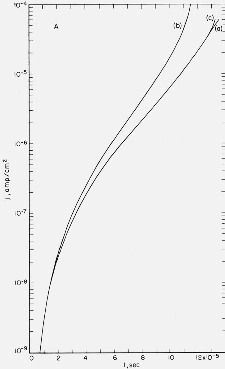
FIGURE 2A. Mean current density  $J$  across the gap versus time  $t$  for  $\gamma_p=0$ ,  $\gamma_i=1.5 \cdot 10^{-5}$ .
