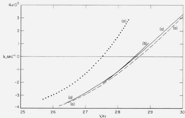
FIGURE 4. Coefficient  $\lambda$  of temporal growth for constant field versus voltage  $V$  across the gap, for  $\Delta x = 0.05$  cm.
