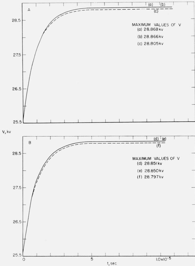
FIGURE 3A. Voltage  $V$  across the gap versus time  $t$  for parameters of figure 2A.
