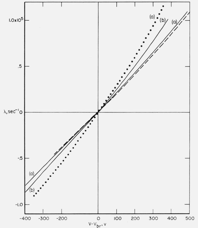
FIGURE 5. Coefficient  $\lambda$  of temporal growth for constant field versus overvoltage  $V - V_{br}$  for same parameters as figure 4.
