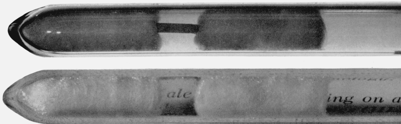
FIGURE 2. Crystal, mounted in quartz tube, diameter 8 mm, with quartz wool packing.
