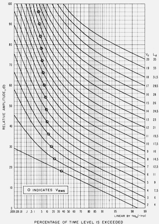
FIGURE 2. Most probable amplitude-probability distribution functions for atmospheric radio noise.
