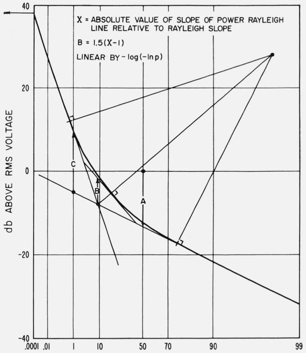
FIGURE 4. Definition of parameters for amplitude-probability distribution for atmospheric radio noise.
