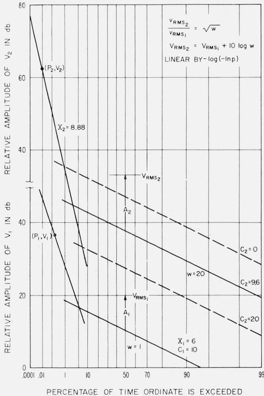
FIGURE 7. The determination of  $C_2$  as a function of  $C_1, X_1,$  and  $w$ .
