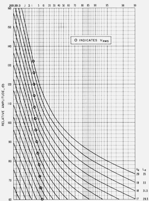
FIGURE 3. Most probable amplitude-probability distribution functions for atmospheric radio noise.
