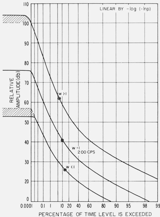
FIGURE 13. Saturation of amplitude-probability distributions for various bandwidths.
