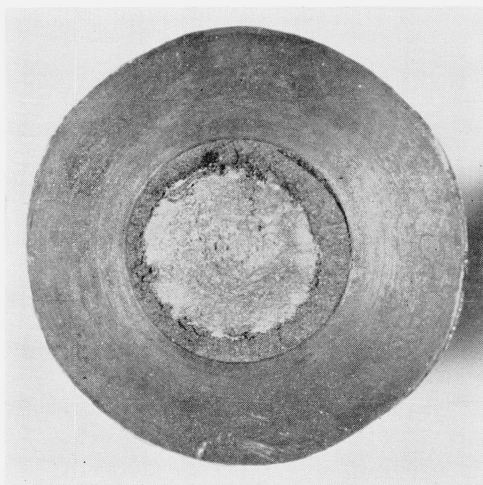
FIGURE 3. Fractured surface of specimen characteristic of that found on specimens from lots B, C and D. \times 4\frac{1}{2} .
