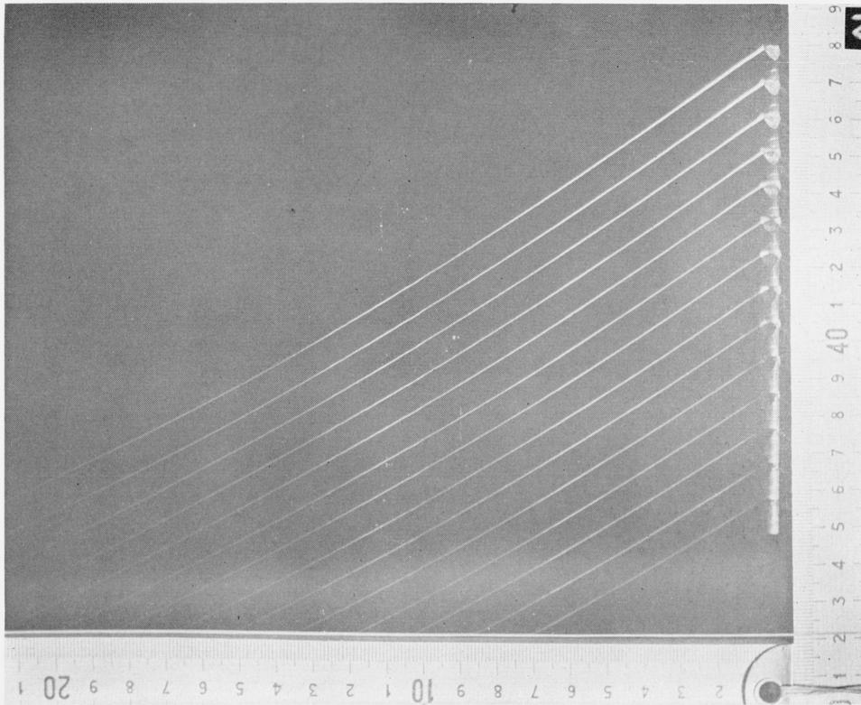
FIGURE 4. Multiflash photograph of a high tenacity nylon yarn struck by a projectile.
