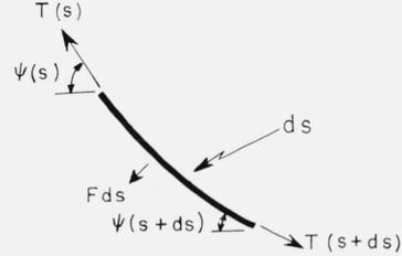
FIGURE 3. A segment  $ds$  of the transverse wave portion of the impacted filament showing tensile forces required to balance the air drag.
