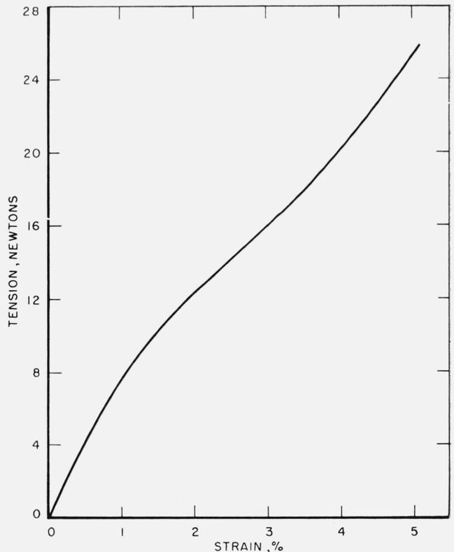
FIGURE 5. Tension-strain curve of high tenacity nylon yarn for a rate of straining of 4800 percent/second.
