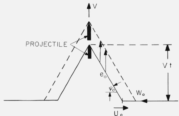
FIGURE 1. Configuration and motion of a filament impacted transversely at velocity  $V$ , air drag neglected.
