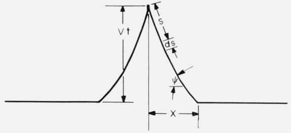
FIGURE 2. Effect of air drag on the shape of a filament impacted transversely at velocity  $V$ .
