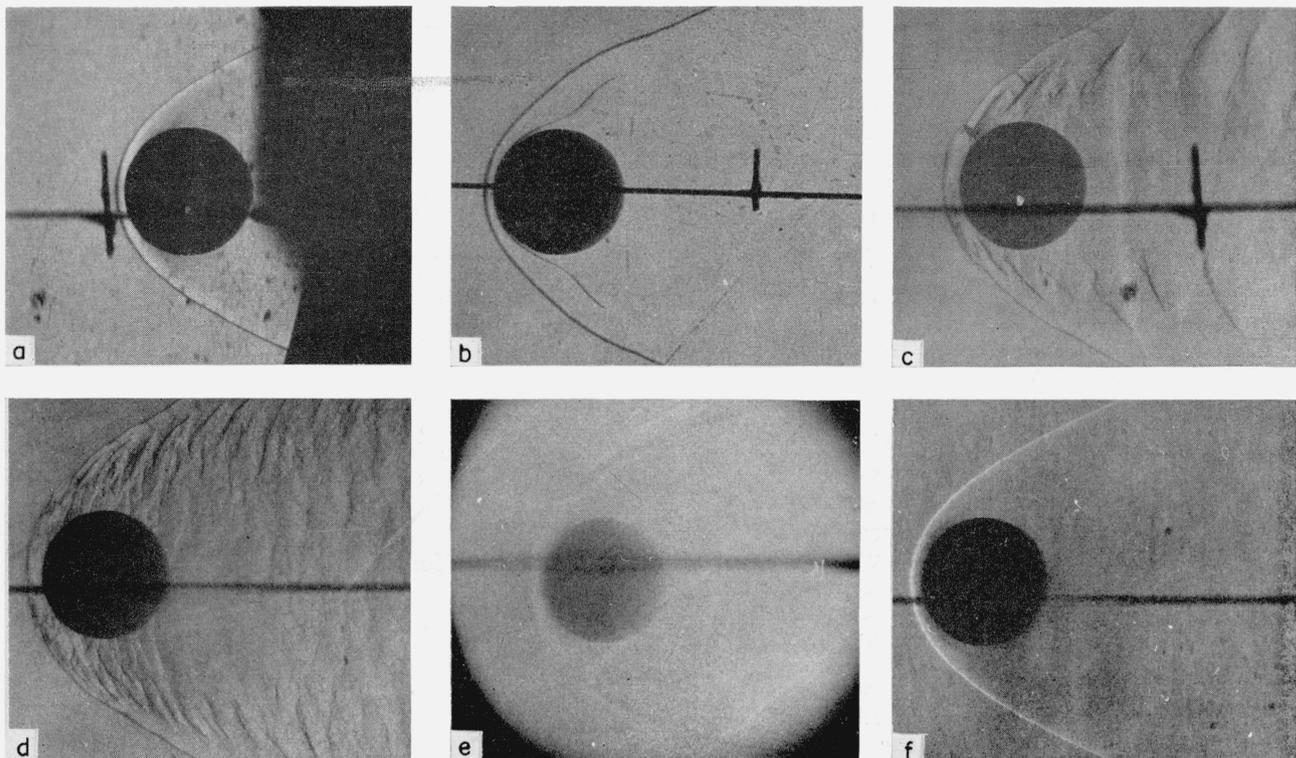
FIGURE 2. *Shadow and schlieren photographs of missile.*
