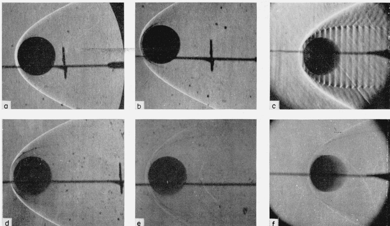
FIGURE 3. *Schlieren photographs of missile,  $p=0.25$  atm.*
