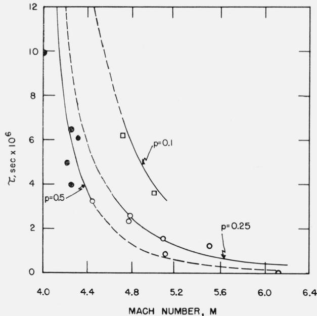
FIGURE 7. Effect of Mach number on ignition delay behind the shock wave.
