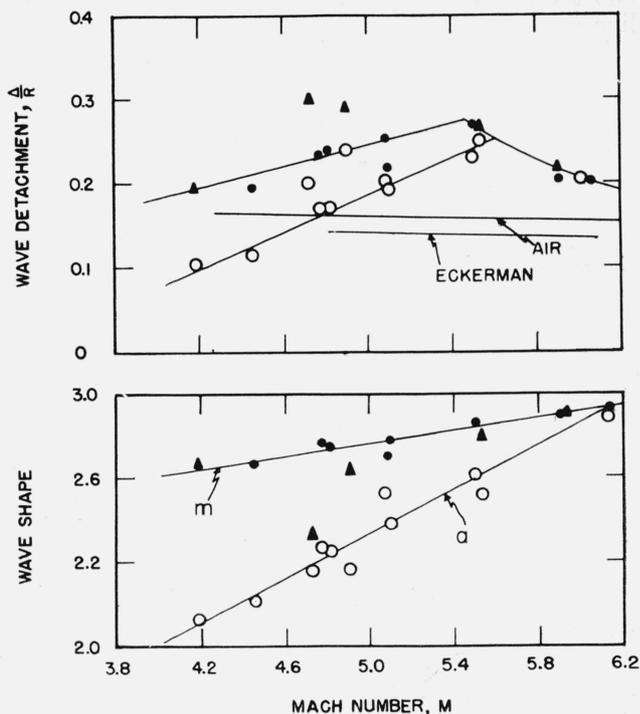
FIGURE 6. Effect of Mach number on wave detachment and shape for a mixture of 30 volume percent  $H_2$  in air at a pressure of 0.25 atm.
