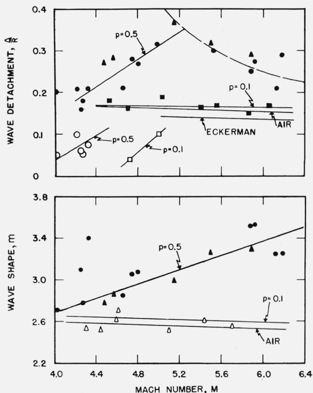
FIGURE 5. Effect of Mach number on wave detachment and shape for a mixture of 30 volume percent  $H_2$  in air at pressures of 0.1 and 0.5 atm.
