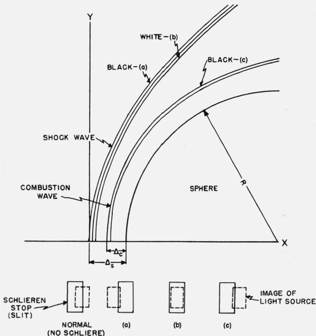
FIGURE 4. Image position of light source for various regions of the schlieren picture and wave coordinate system.
