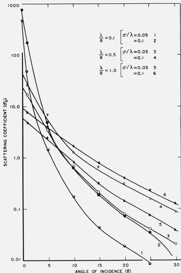
FIGURE 4. Scattering coefficient versus the angle of incidence.
