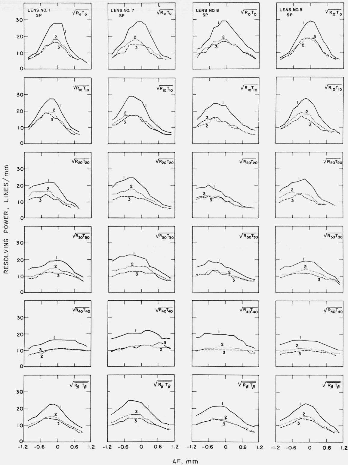
FIGURE 2. Average resolving power versus position of the image plane for four lenses with SP emulsion.
