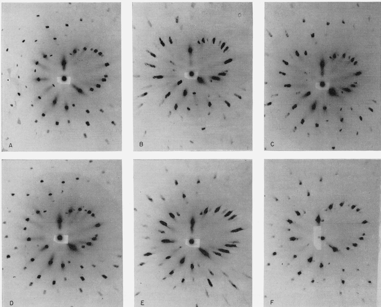
FIGURE 1. Set of transmission Laue patterns of large aluminum grain in specimen bent through  $\frac{1}{4}$  cycles of plastic deformation. A. Annealed (zero position); B. positive bending; C. zero position; D. negative bending; E. zero position; F. positive bending.
