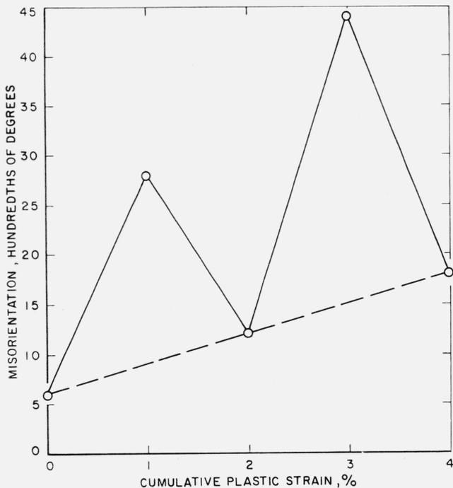
FIGURE 6. Average misorientation versus cumulative strain for one cycle of plastic strain of 1 percent amplitude.
