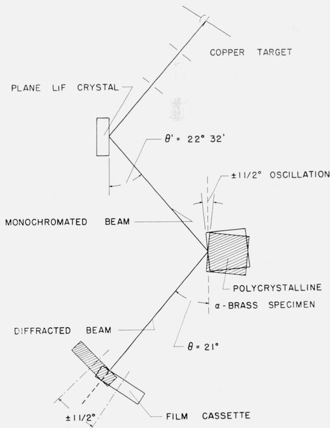
FIGURE 3. Schematic diagram of the monochromatic misorientation goniometer.
