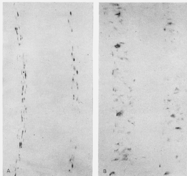
FIGURE 5. A pair of patterns made with the monochromatic misorientation goniometer with Cu  $K\alpha$  radiation showing the (111) and (200) diffractions from brass, which had been extended 1 percent.
