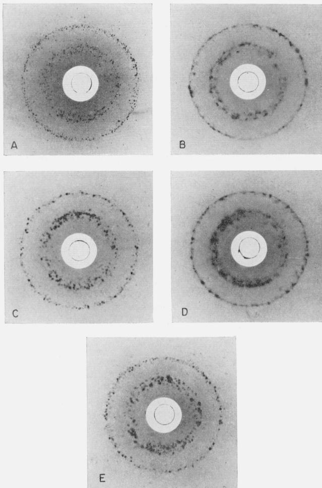
FIGURE 2. High-angle X-ray diffraction patterns from copper rod at stages in one cycle of torsion.
