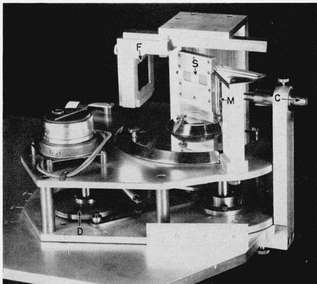
FIGURE 4. Photograph of the monochromatic misorientation goniometer.
