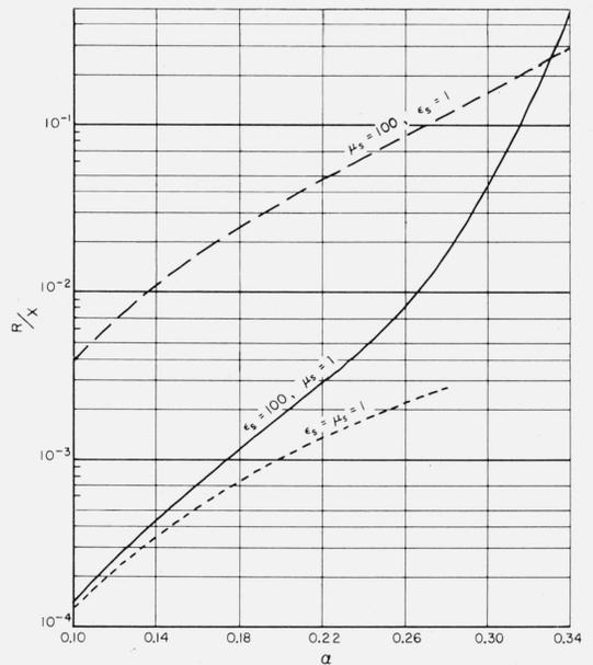
FIGURE 5. Ratios of radiation resistances to radiation reactances of uniform current loops having air, dielectric, and magnetic cores ( $N=1, 10$ ;  $a/b=60$ ).
