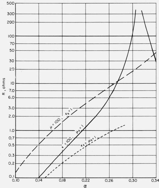
FIGURE 3. Radiation resistances of uniform current loops having air, dielectric, and magnetic cores ( $N=1, 10$ ;  $a/b=60$ ).
