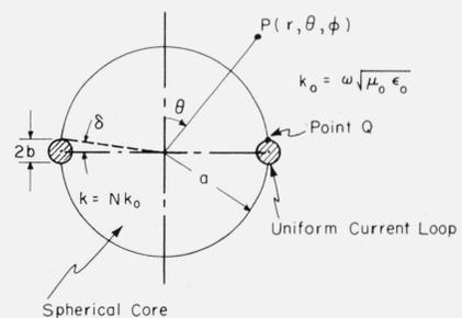
FIGURE 1. Uniform current loop having a spherical core.
