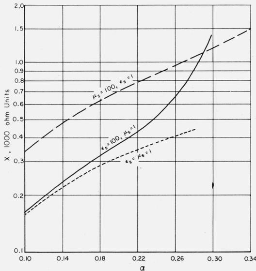
FIGURE 4. Radiation reactances of uniform current loops having air, dielectric, and magnetic cores ( $N=1, 10$ ;  $a/b=60$ ).
