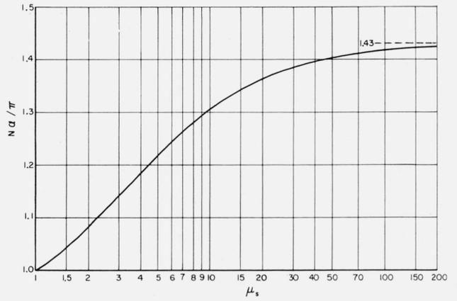
FIGURE 2. Antiresonance frequency of a uniform current loop having a spherical core with arbitrary constants  $\mu_s$  and  $\epsilon_s$ , where  $N\alpha = \sqrt{\mu_s \epsilon_s} k_0 a = ka$ .
