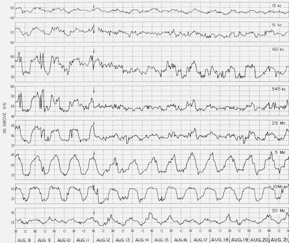
FIGURE 3. Radio noise power recorded at Kekaha, Hawaii: August 8 to August 21, 1958. Time of explosion indicated by arrows.
