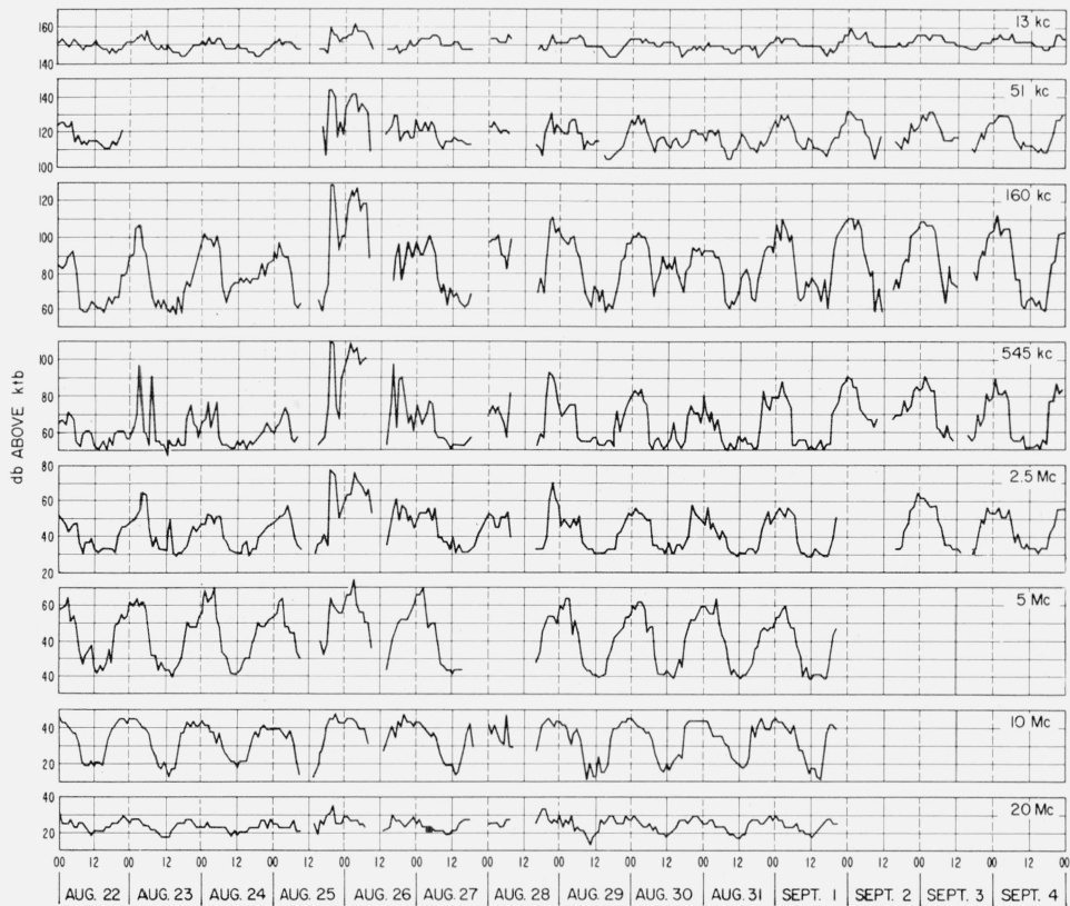
FIGURE 4. Radio noise power recorded at Kekaha, Hawaii: August 22 to September 4, 1958.
