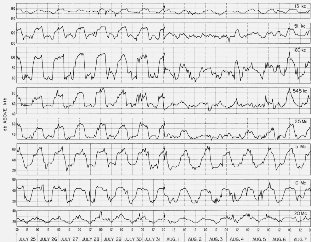
FIGURE 2. Radio noise power recorded at Kekaha, Hawaii: July 25 to August 7, 1958.
