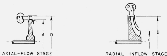
FIGURE 3. Typical radial and axial flow stages.
