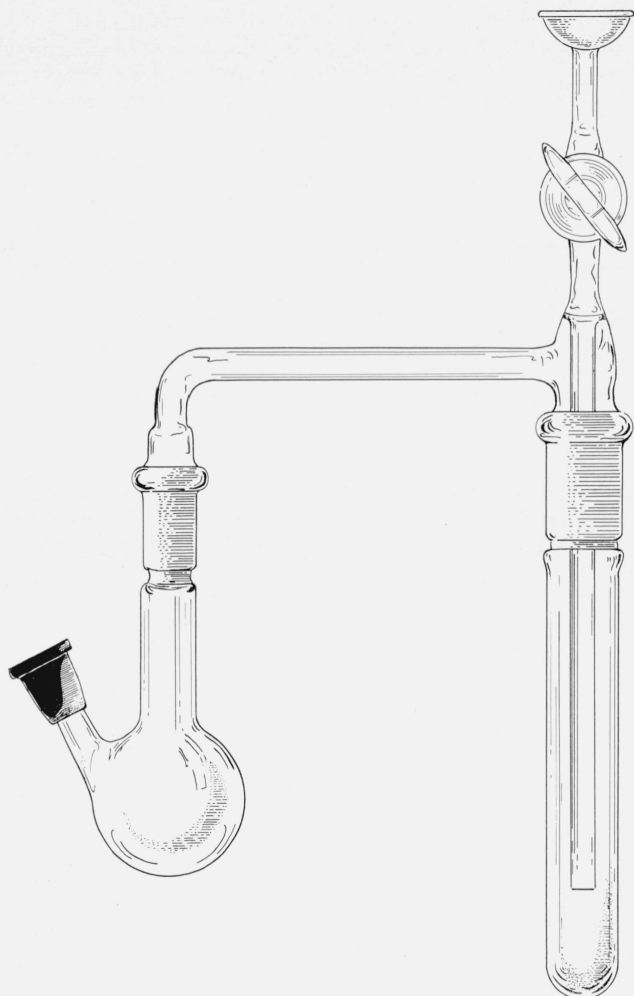
FIGURE 1. Apparatus for conducting reductions with lithium borohydride- t .
