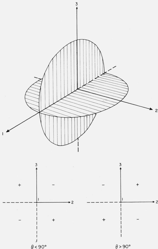
FIGURE 7. How the sign of the correlation is governed by the direction of the antenna axis.
