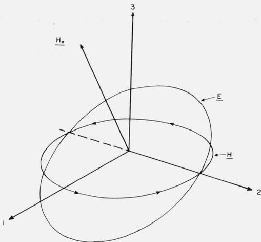
FIGURE 3. The polarization of waves in the whistler mode.
