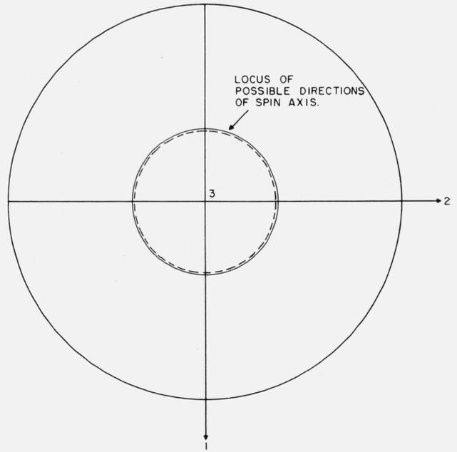
FIGURE 9. The possible directions of the spin axis, for a given value of  $|\cos \Psi|$ .
