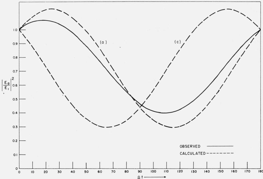
FIGURE 11. Comparison of the "observed" and calculated variations of the strength of the electric signal; in the calculations, it was assumed that  $\theta = 150^\circ$ .
