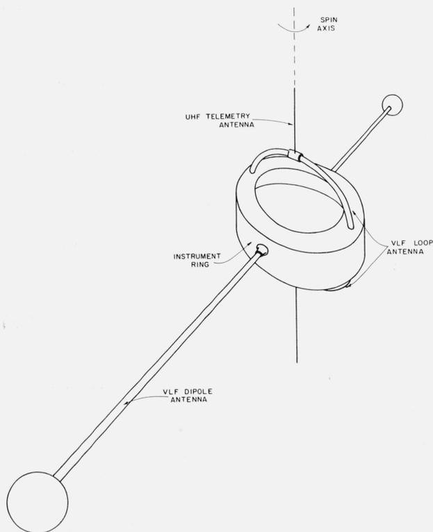
FIGURE 4. The mechanical design of the satellite (the outer cover is not shown).
