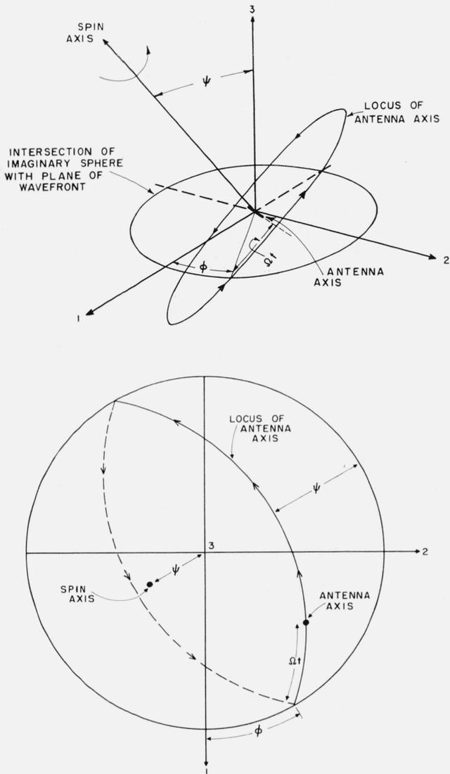
FIGURE 6. The geometry of the spinning motion.
