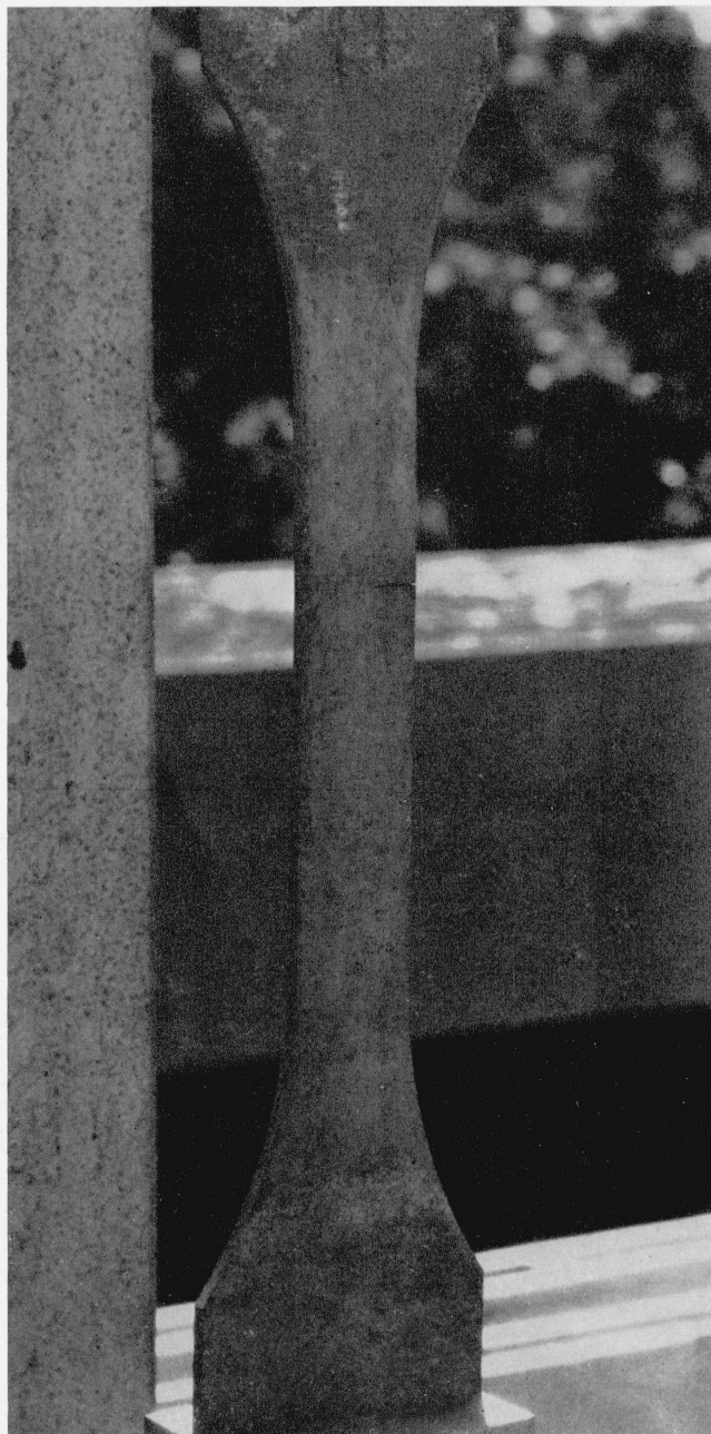
FIGURE 3. Specimen exposed to weather at NBS. Note stress-corrosion crack extending about \frac{1}{3} through specimen.
