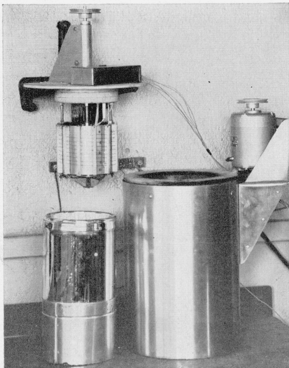
FIGURE 2. Adiabatic furnace, showing Dewar flask and specimen container removed from insulating shell.
