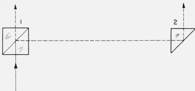
FIGURE 3. The elements of a superimposed-image range finder.
