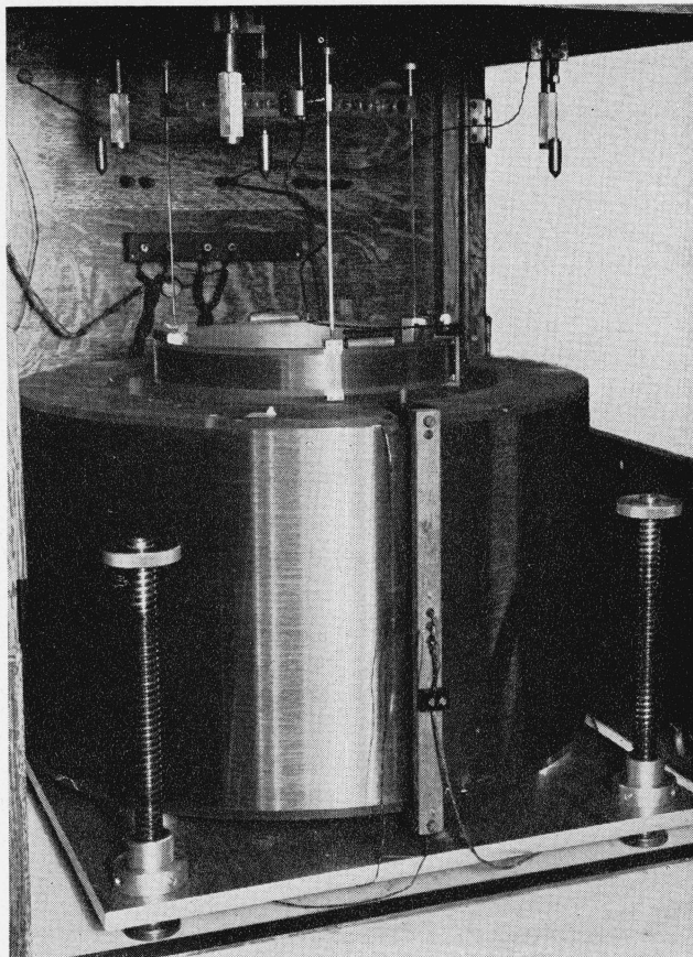
FIGURE 3. Coil case with fixed coil lowered to show movable coil.
