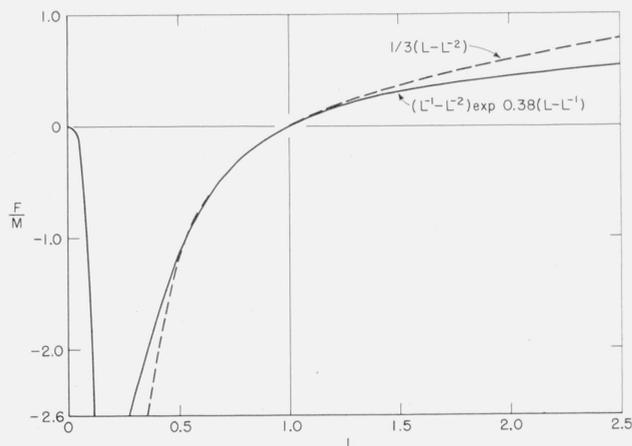
FIGURE 1. Relation between stress-modulus ratio  $F/M$  and length ratio  $L$ .
