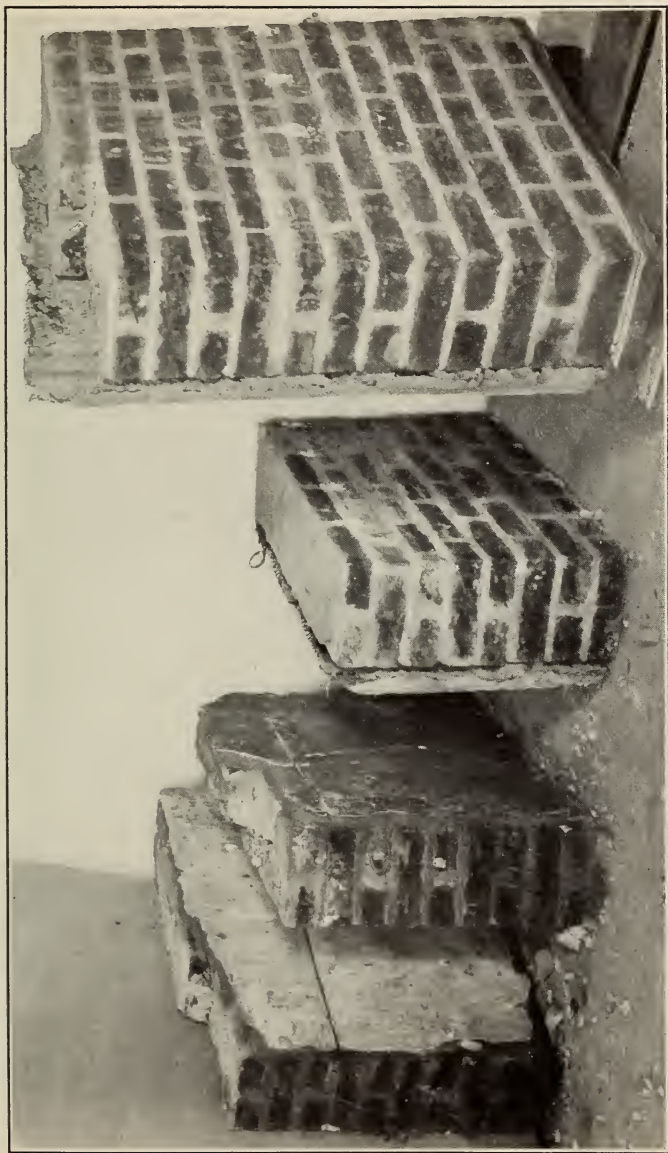
FIGURE 6.—View of brick walls Nos. 1 and 6 after test, showing character of workmanship
