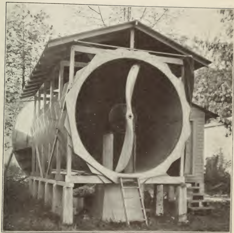
FIGURE 1.—Test duct with inlet ring removed and 9-foot 11-inch fan in place
