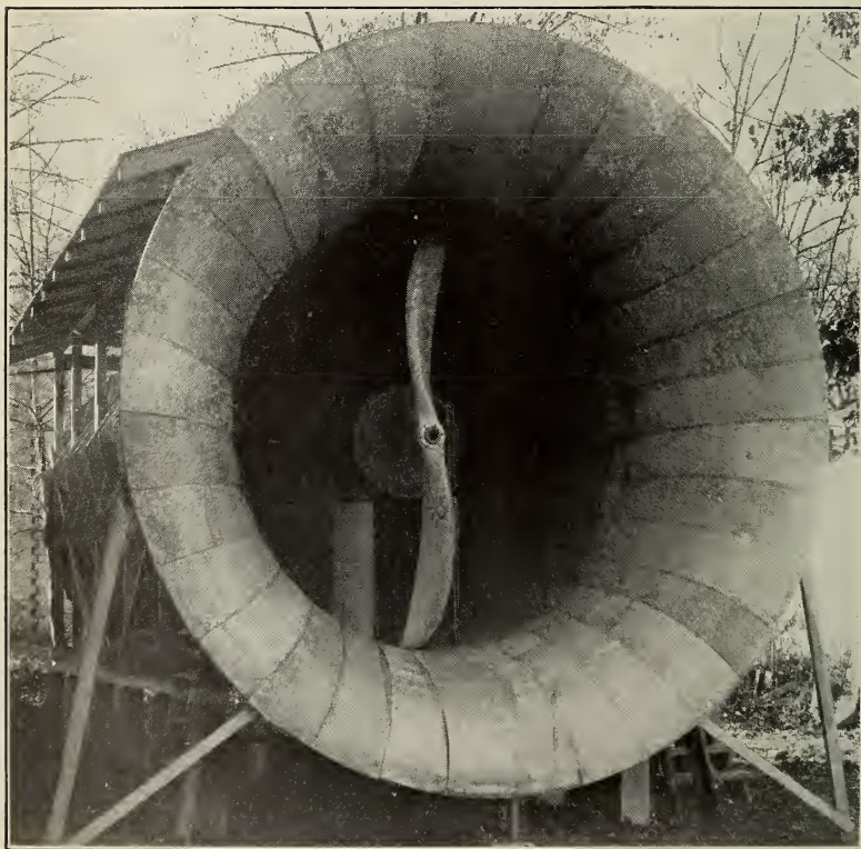
FIGURE 2.— Test duct with faired entrance section for blower condition
