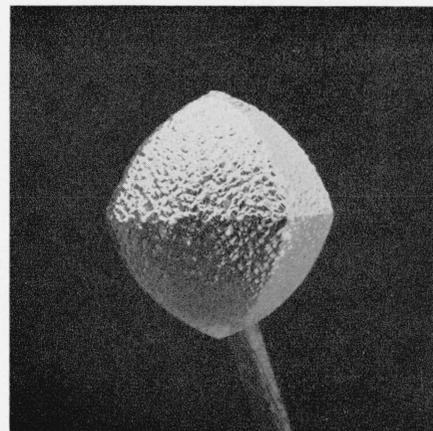
FIGURE 16. Monocrystalline aluminum sphere deeply corroded in an aqua regia-HF mixture. ×2.
