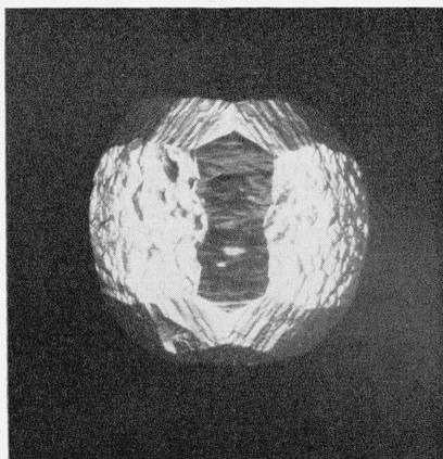
FIGURE 26. *Monocrystalline aluminum sphere corroded in 15-percent NaOH.*
