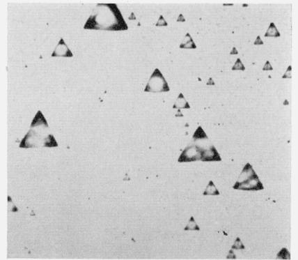
FIGURE 14. Photomicrograph of etched surface of monocrystalline aluminum approximately parallel to (111).
