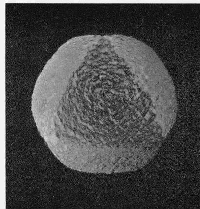
FIGURE 30. *Deeply corroded version of sphere shown in figure 8.*
