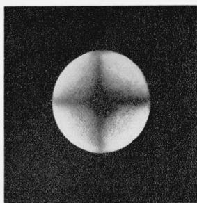
FIGURE 6. Monocrystalline aluminum sphere after corrosion in aqua regia-HF solution.
