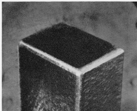
FIGURE 23. Rectangular parallelepiped with six faces parallel to cubic planes after exposure to an aqua regia-HF mixture.  $\times 3$ .
