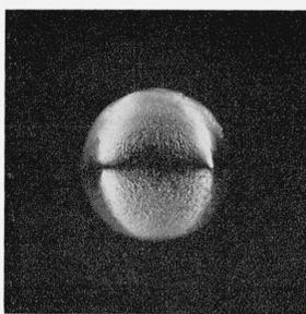
FIGURE 7. Monocrystalline aluminum sphere after corrosion in aqua regia-HF solution.
