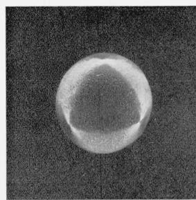
FIGURE 8. Monocrystalline aluminum sphere after corrosion in aqua regia-HF solution.
