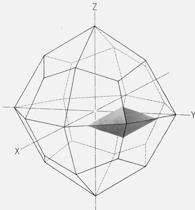
FIGURE 40. Sketch of tetragonal trisoctahedron showing hillock as viewed in a direction normal to the dodecahedral plane.
