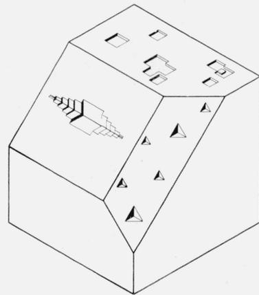
FIGURE 15. Sketch of cube showing etch pits bounded by cubic planes on cubic, dodecahedral, and octahedral faces.
