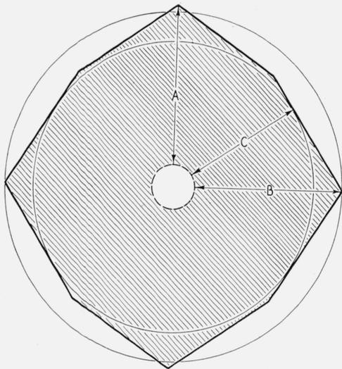
FIGURE 32. Sketch of hole in disk whose surface is parallel to dodecahedral plane after corrosion in 15-percent NaOH.
