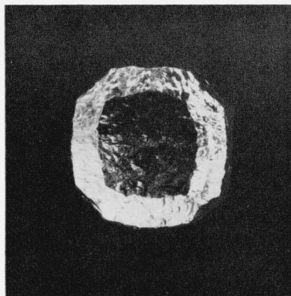
FIGURE 25. *Monocrystalline aluminum sphere corroded in 15-percent NaOH.*
