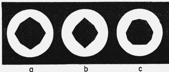
FIGURE 36. *Shadow photographs of tetragonal trisoctahedron having sides parallel to  $\{335\}$ .*
