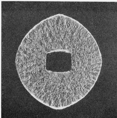
FIGURE 18. Disk with surface parallel to dodecahedral plane after corrosion in aqua regia-HF solution.
