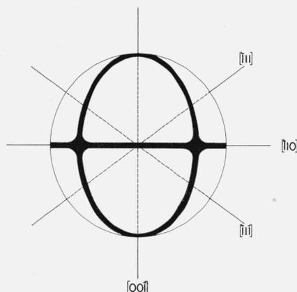
FIGURE 4. Sketch of sphere shown in figure 7, oriented with the dodecahedral plane parallel to the paper and showing loci of cubic, dodecahedral, and octahedral directions.
