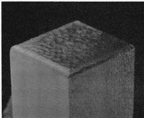
FIGURE 24. Rectangular parallelepiped with two faces parallel to cubic planes and four faces parallel to dodecahedral planes after exposure to an aqua regia-HF mixture.  $\times 3$ .
