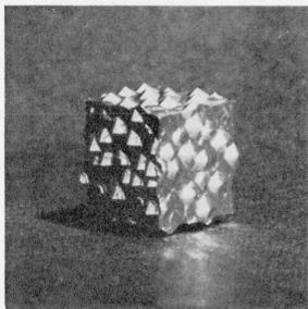
FIGURE 33. Cube with six faces parallel to  $\{100\}$  after exposure to a 15-percent NaOH solution.  $\times 1\frac{1}{2}$ .
