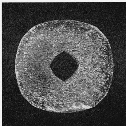
FIGURE 21. Disk with surface parallel to dodecahedral plane after corrosion in 15-percent NaOH solution.
