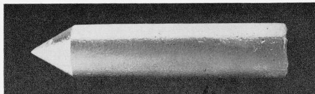
FIGURE 11. Aluminum monocrystal used for machining of specimens.  $\times \frac{1}{2}$ .
