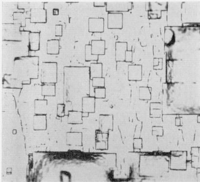
FIGURE 12. Photomicrograph of etched surface of monocrystalline aluminum approximately parallel to (100).
