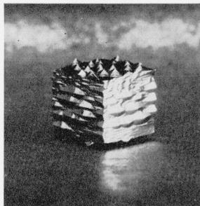
FIGURE 34. Cube with two faces parallel to  $\{100\}$  and four faces parallel to  $\{110\}$  after exposure to 15-percent NaOH solution.  $\times 1\frac{1}{2}$ .
