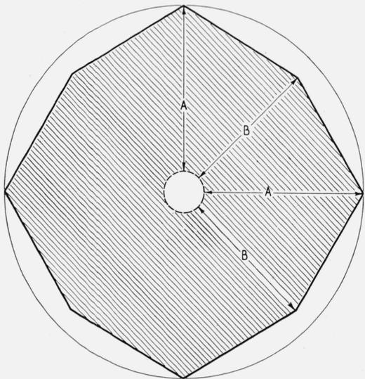
FIGURE 31. Sketch of hole in disk whose surface is parallel to cubic plane after corrosion in 15-percent NaOH.
