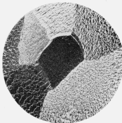
FIGURE 1. High-purity, polycrystalline aluminum deep-etched in an aqua regia-HF solution.  $\times 3$ .
