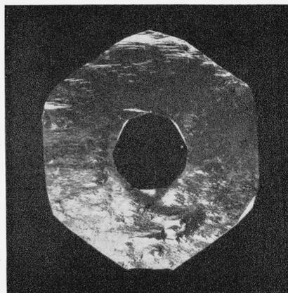
FIGURE 22. Disk with surface parallel to octahedral plane after corrosion in 15-percent NaOH solution.
