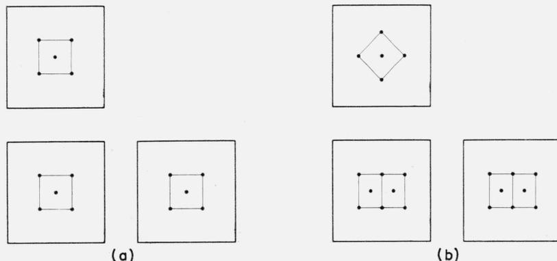
FIGURE 10. Orthographic projections of cubes having faces parallel to cubic and dodecahedral planes and showing the unit-cell arrangement when viewed in directions normal to these planes.
