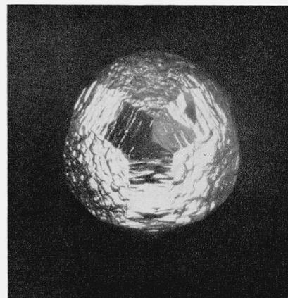
FIGURE 27. *Monocrystalline aluminum sphere corroded in 15-percent NaOH.*
