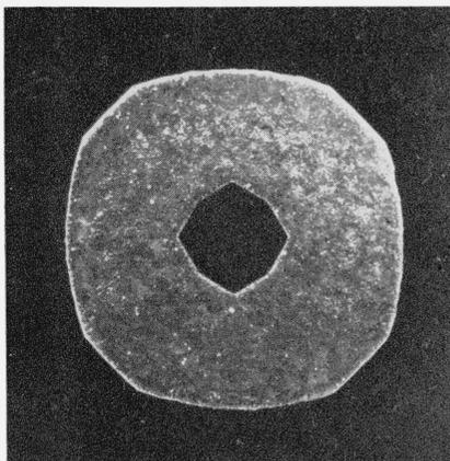
FIGURE 20. Disk with surface parallel to cubic plane after corrosion in 15-percent NaOH solution.
