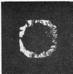
FIGURE 37. *Corroded sphere shown in figure 25 after longer exposure to 15-percent NaOH.  $\times 3$ .*
