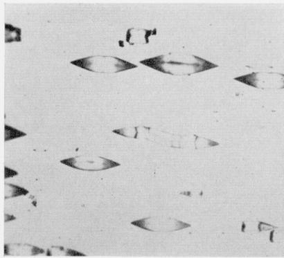
FIGURE 13. Photomicrograph of etched surface of monocrystalline aluminum approximately parallel to (110).
