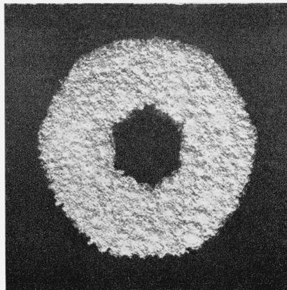
FIGURE 19. Disk with surface parallel to octahedral plane after corrosion in aqua regia-HF solution.
