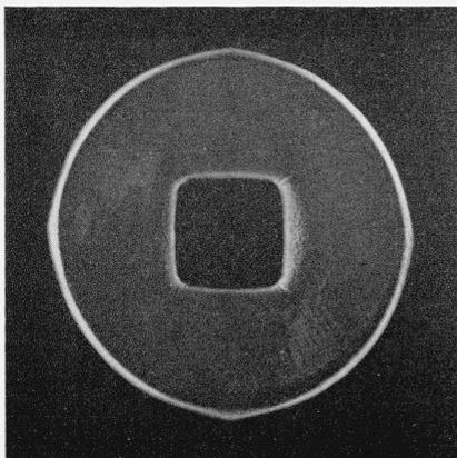
FIGURE 17. Disk with surface parallel to cubic plane after corrosion in aqua regia-HF solution.
