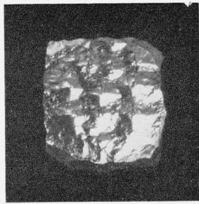
FIGURE 38. *Corroded sphere shown in figure 37 after still longer exposure to 15-percent NaOH.  $\times 5$ .*
