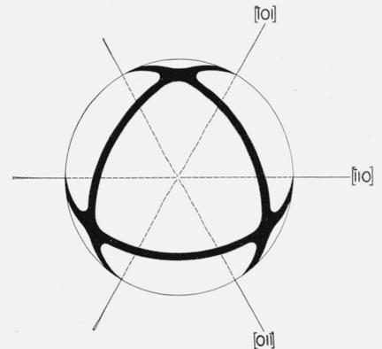
FIGURE 5. Sketch of sphere shown in figure 8, oriented with the octahedral plane parallel to the paper and showing loci of the dodecahedral directions.
