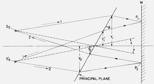
FIGURE 2. Ray trace through the interferometer.
