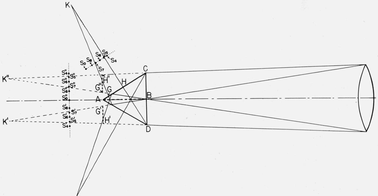
FIGURE 4. Relative positions of source, prism, and lens (or mirror) for various types of interferograms.
