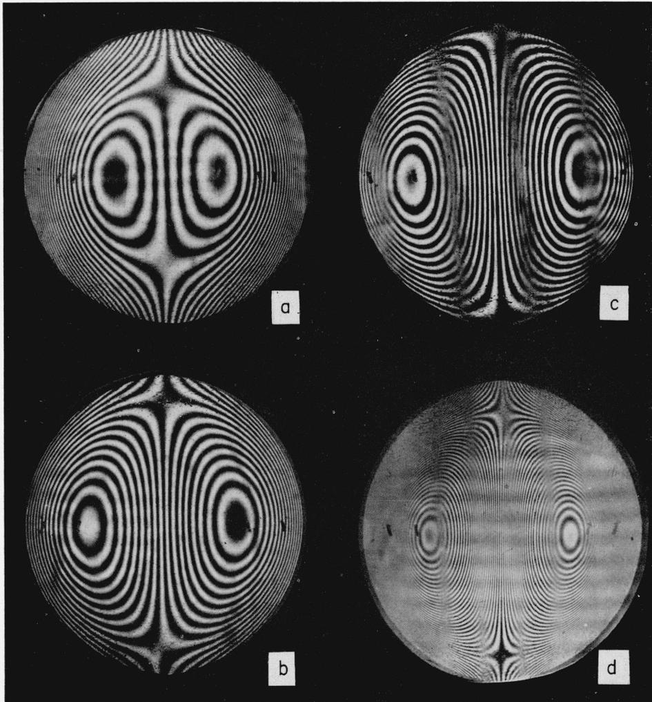
FIGURE 3. Interferograms with the Kösters double-image prism.
