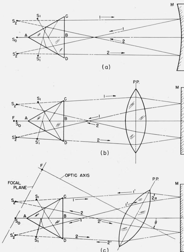
FIGURE 1. The Kösters prism and lens interferometer.
