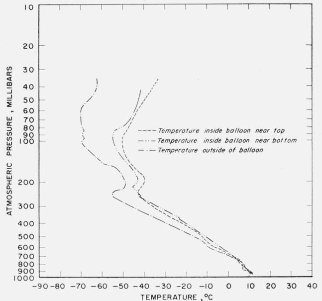
FIGURE 6. *Temperatures inside and outside of a post-plasticized balloon during a day flight.*
