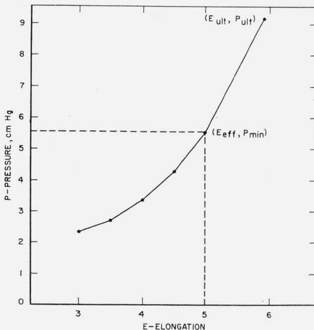
FIGURE 3. Differential pressure versus elongation in patch tests at  $-60^\circ$  C.
