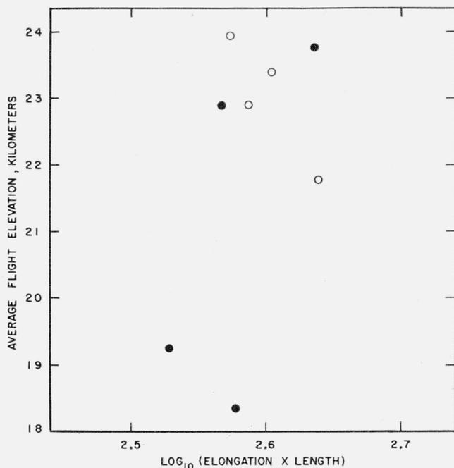
FIGURE 5. Correlation between flight elevation and ultimate elongation.
